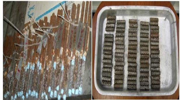
Figure 4: Samples of corroded rebars before and after cleaning.
