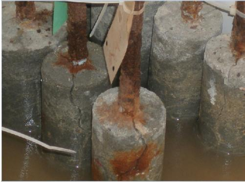
Figure 3: Sample of test-specimens exposed to chloride solution.
