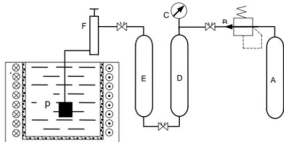
**Figure 1.** The schematic diagram of flotation equipment
