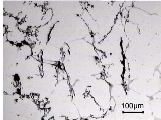
**Figure 5.** Oxide inclusion in A356 cast alloy
