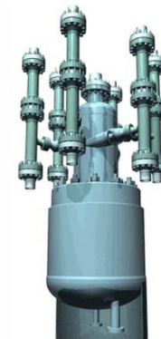
Separation of hydrates from gas/liquid streams
