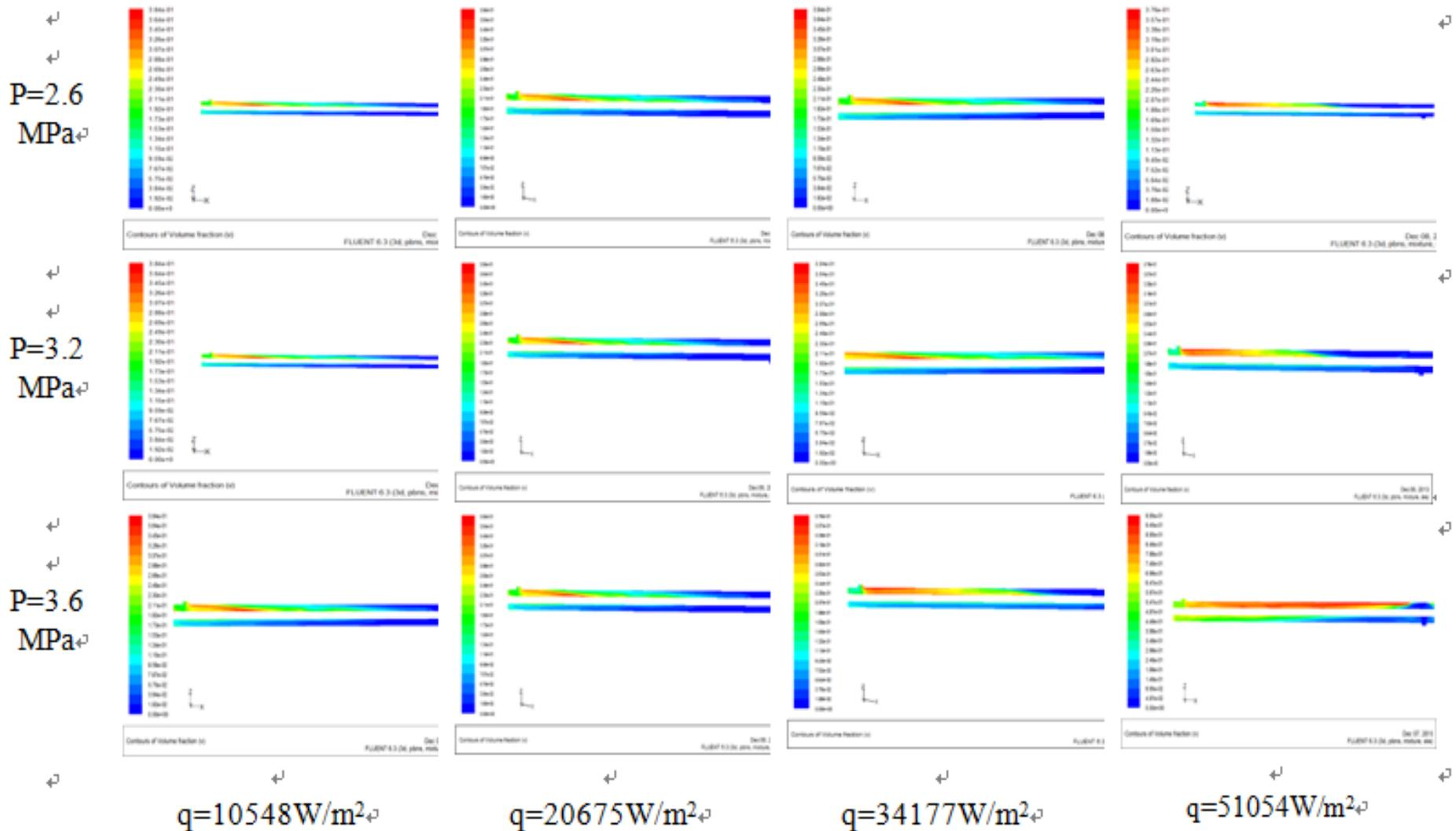
**Figure 4:** Contours of volume fraction under different pressure and heat flux
