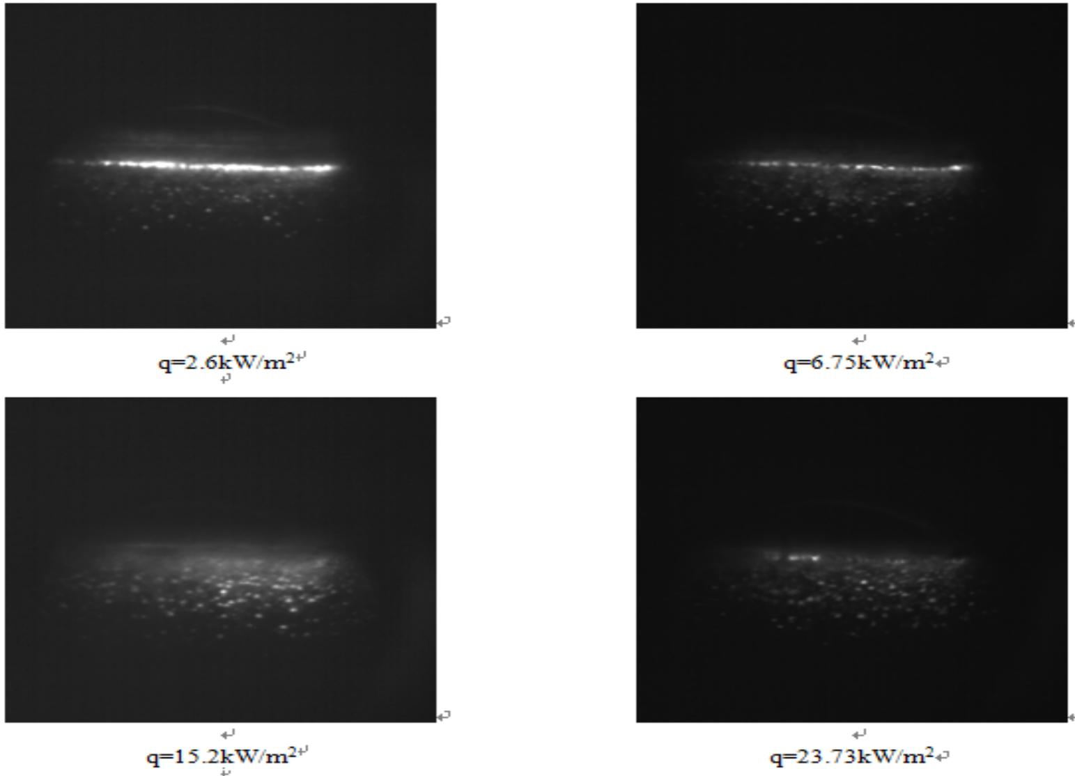
**Fig. 5** : CO<sub>2</sub> pool boiling images at 3.6 MPa under different heat flux density
