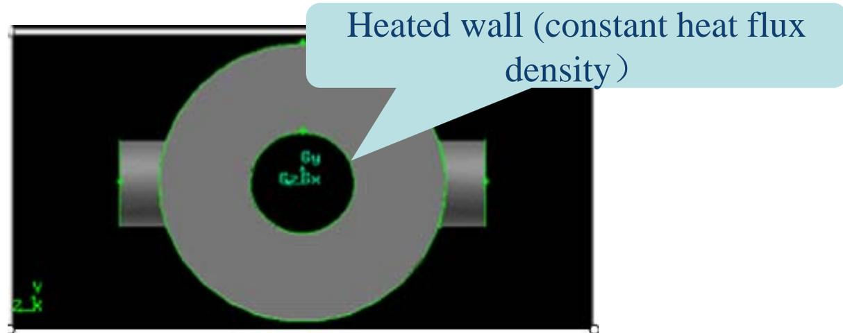
**Figure 3:** Vertical model of test section
