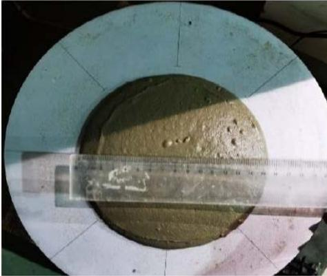
Figure 1. The measurement of flow value
