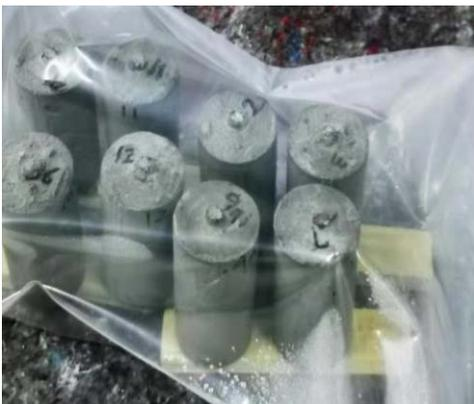
Figure 3. Sealed curing
