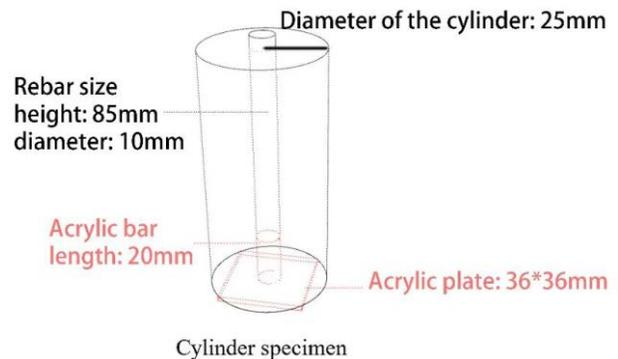
Figure 4. The cylinder specimen for accelerated corrosion test
