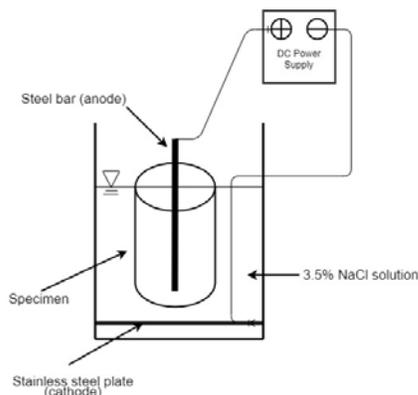
**Figure 5.** Schematic view of impressed current setup
