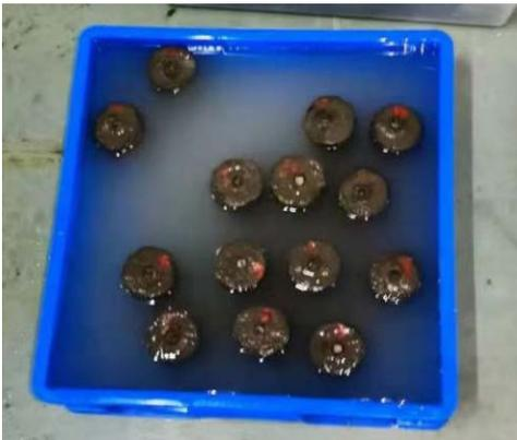
Figure 2. Submerged curing
