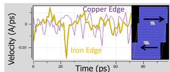
Edge Velocities<sup>[3]</sup> – Dislocation cores move at roughly constant value for constant shear rate
