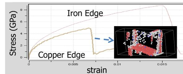
Fixed Strain Rate and Temperature<sup>[3]</sup> – Different magnitudes because dislocations in Copper are partials compared to Iron. Inset shows an example nucleation event at high strain
