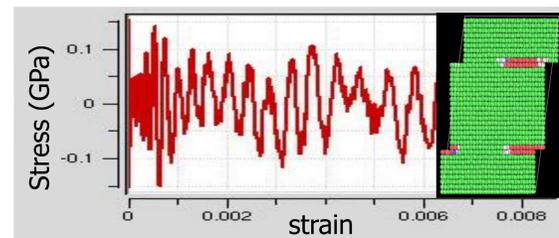
Edge Dislocation FCC Copper<sup>[3]</sup> – Oscillation around 0 GPa conveys gliding motion
