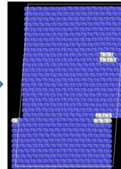
Final state of the simulation where the applied shear moves the dislocation. Defects are created and simulated using the LAMMPS<sup>[4]</sup> simulation package.
