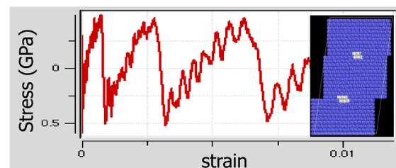
Edge Dislocation BCC Iron<sup>[3]</sup> – Increasing stress implies single dislocation takes more stress to move than two partials in a FCC crystal
