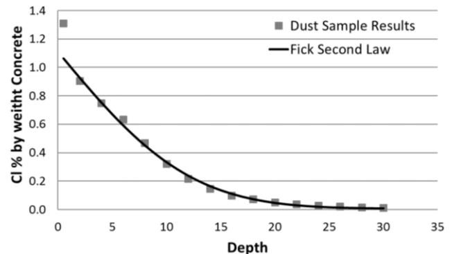
**Fig. 4.** OPC chloride profile with Fick's law fitted
