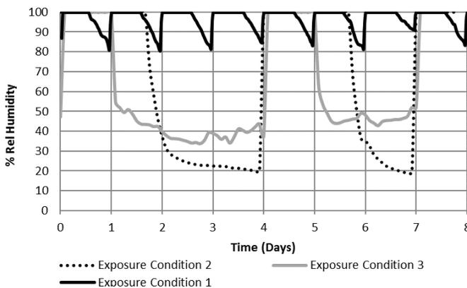
**Fig. 1.** Relative humidity plot showing weekly cycle for three exposure conditions
