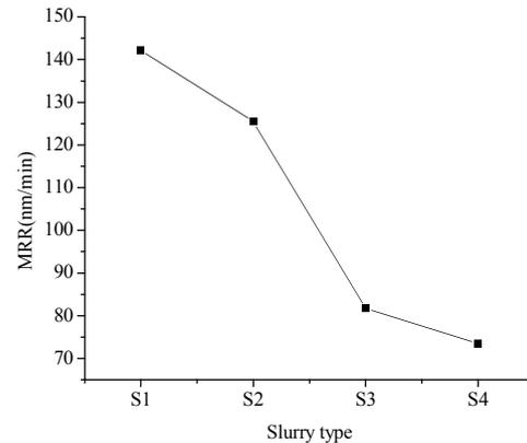
**Fig. 2** MRR of the four slurries
