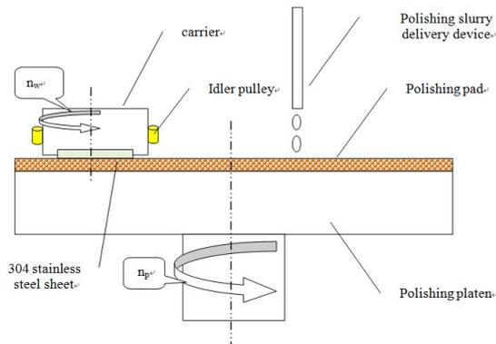
Fig.1 The schematic of CMP system
