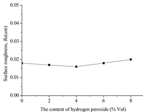
Fig.7 Surface roughness of the content of hydrogen peroxide
