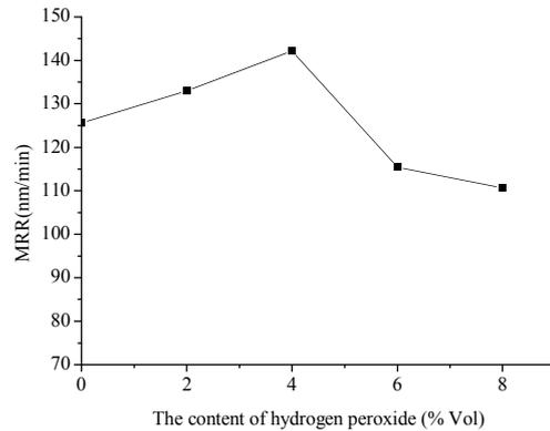
Fig.6 MRR of the content of hydrogen peroxide
