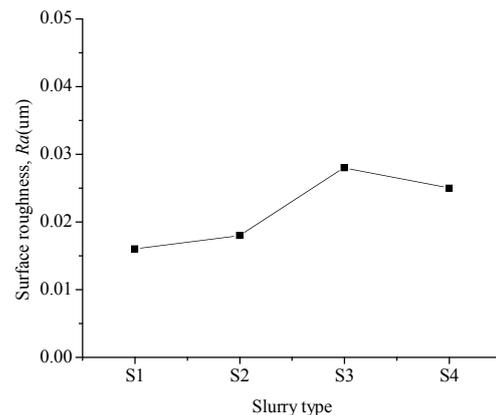
**Fig. 3** Surface roughness after CMP using the four slurries
