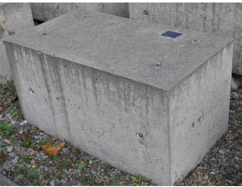
**Fig. 13.** Condition of exposure block NMLiN1.25 after 15 years outdoors (0.041% expansion).
