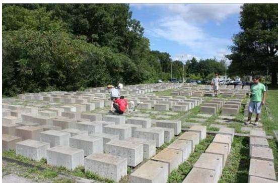
**Fig. 1.** Concrete blocks disposed on the CANMET outdoor exposure site.
