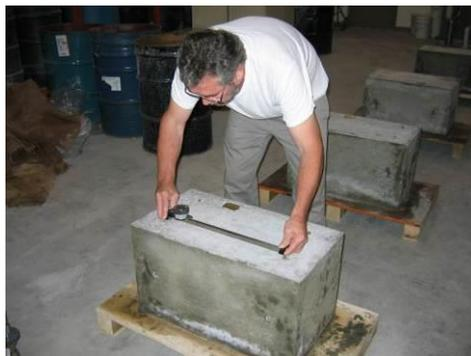
**Fig. 3.** Measurement on the longitudinal axis on the top of a concrete block (gage length is 500mm).
