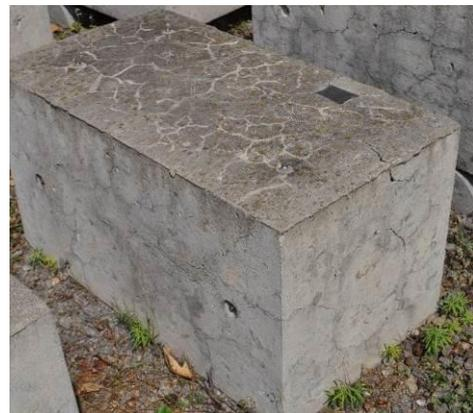
**Fig. 9.** Condition of control exposure block NM after 15 years outdoors (0.684% expansion).
