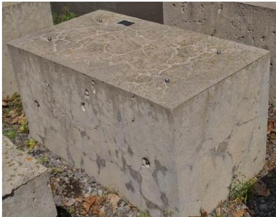
**Fig. 18.** Condition of control exposure block Wy+ after 15 years of storage outdoors (0.295% expansion).
