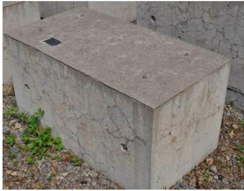
**Fig. 12.** Condition of exposure block NMLiN1.0 after 15 years outdoors (0.355% expansion).
