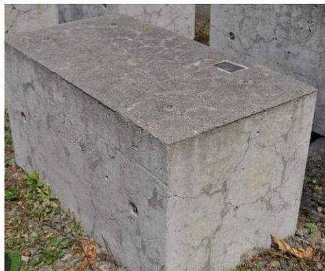
**Fig. 10.** Condition of exposure block NMLiOH1.0 after 15 years outdoors (0.390% expansion).
