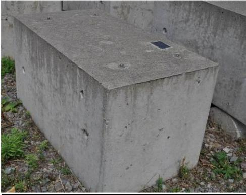
**Fig.11.** Condition of exposure block NMLiOH1.5 after 15 years outdoors (0.034% expansion).
