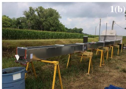
Figures 1(a) and 1(b): 20- flume and 10-m flume used in the instantaneous and constant injections, respectively.
