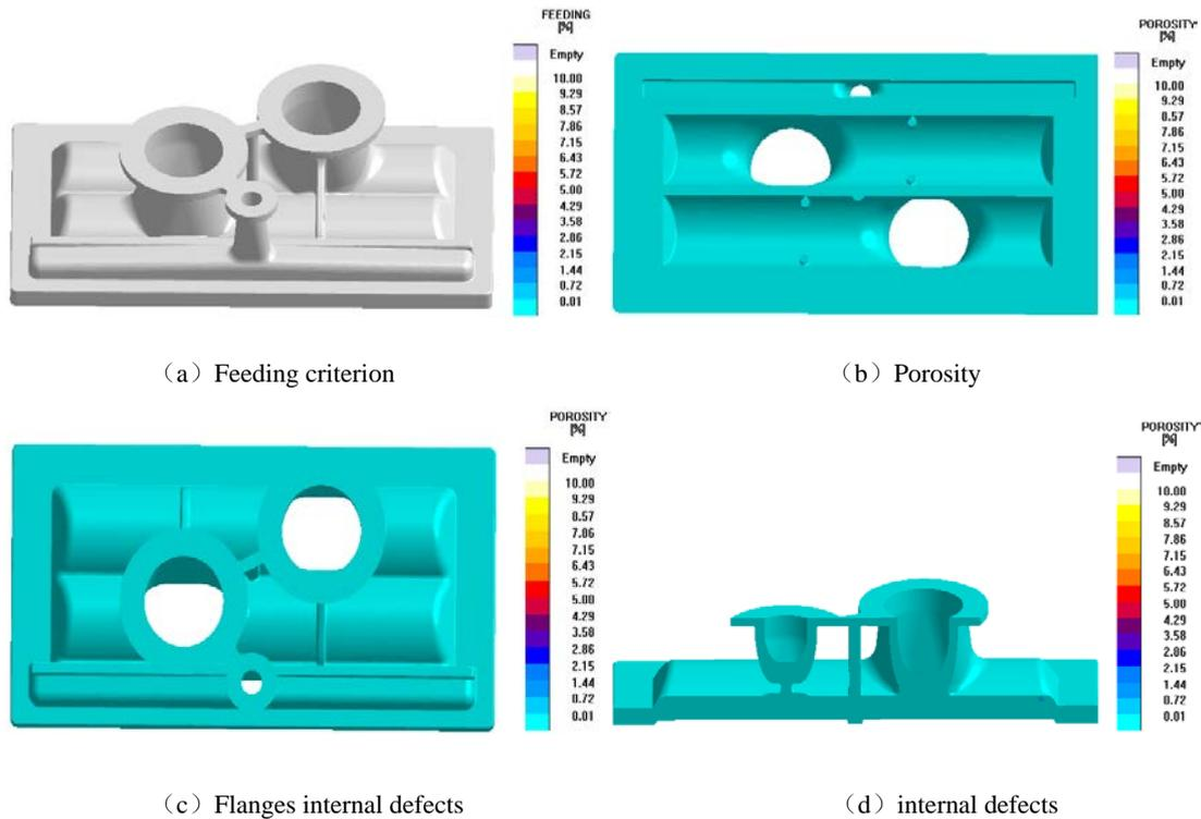
Fig.9 Shrinkage criterion
