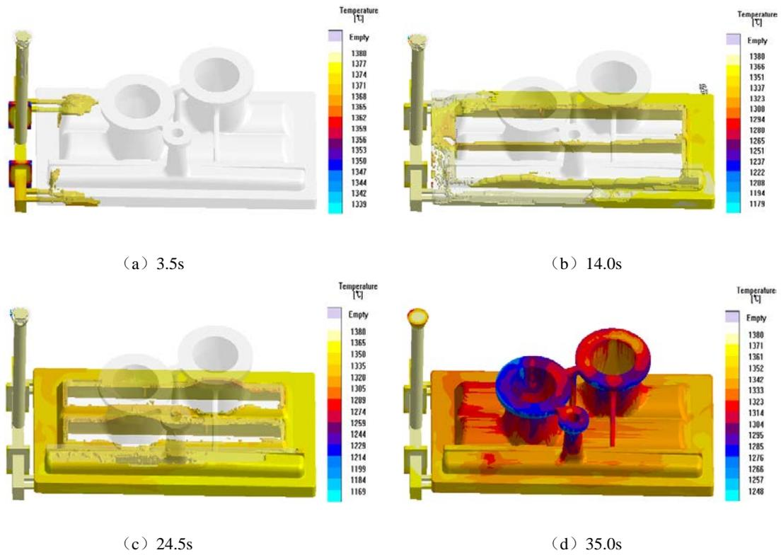
Fig.7 filling process of the casting process
