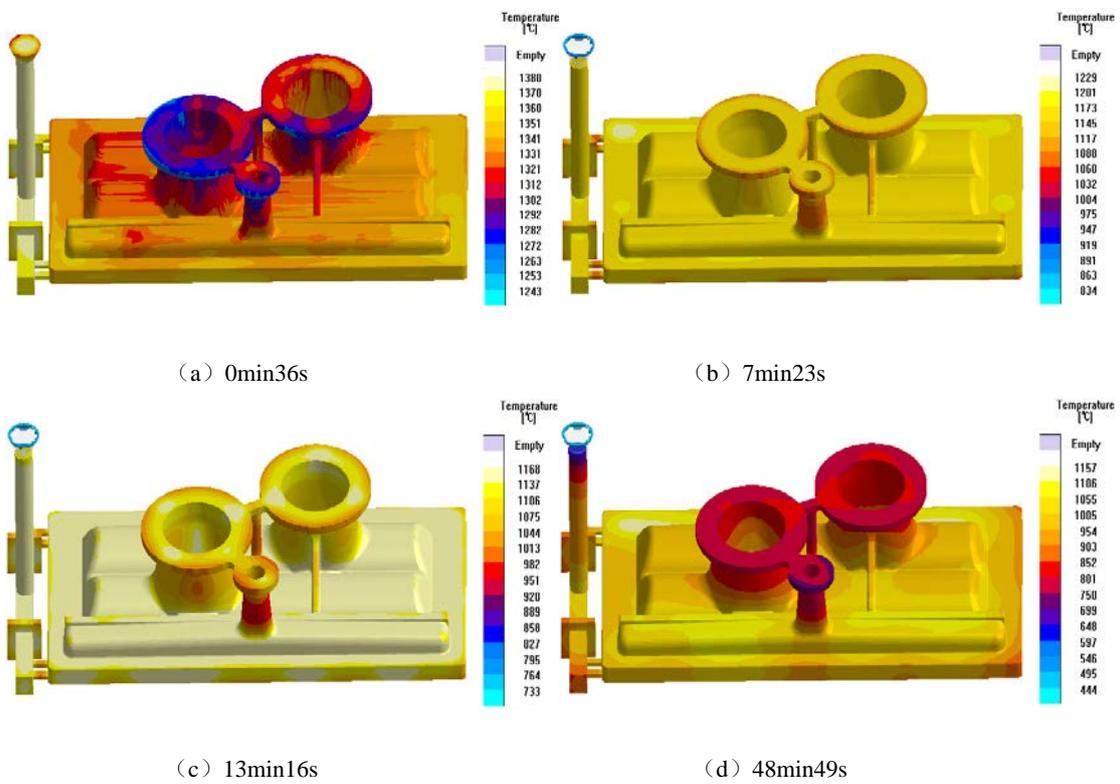
Fig.8 the solidification process of the casting
