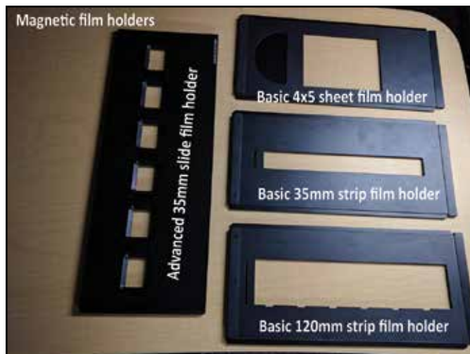
Figure 4: Magnetic Holders for Digitalization of Transparencies
