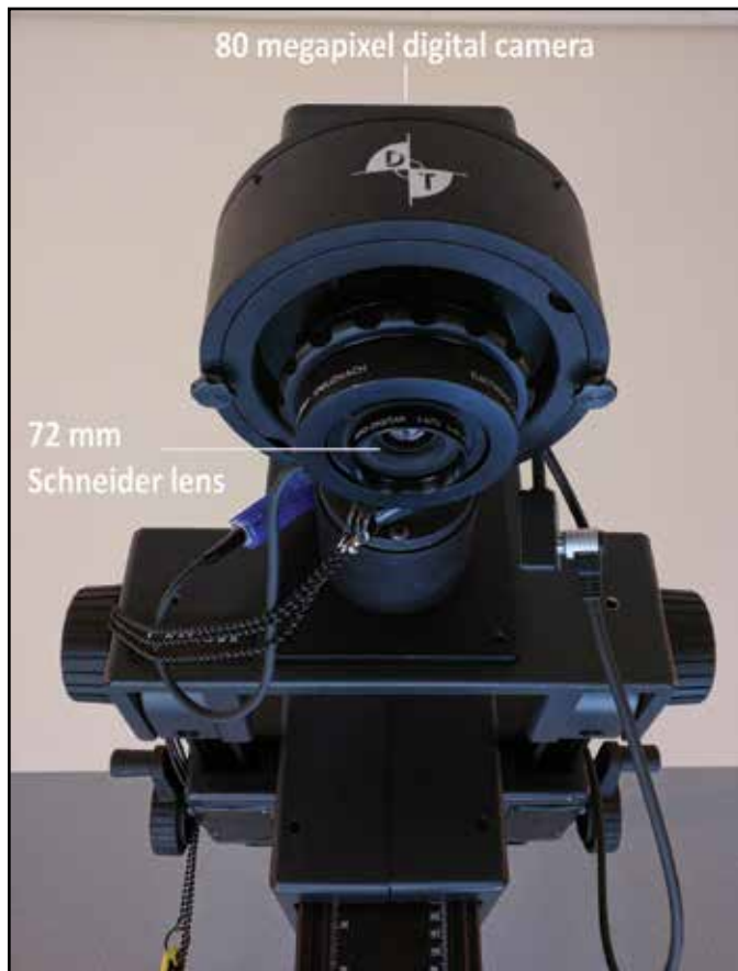
Figure 2: Phase One Camera Set Up with 72Mm Schneider Lens
