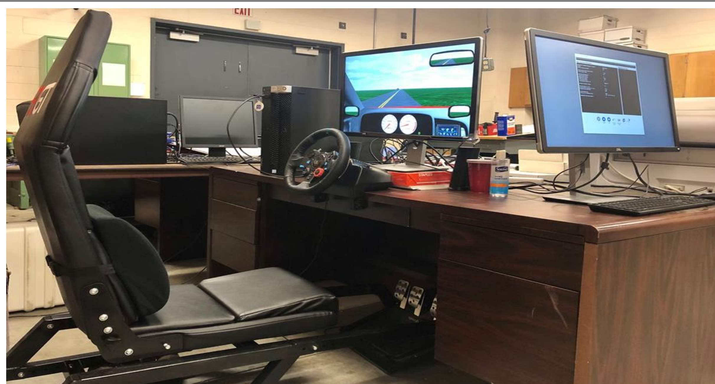
Figure 1. Driving Simulator and Eye Tracker System
