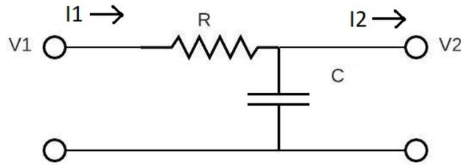
**Figure 1:** The two-port matrix representation of an RC Circuit
