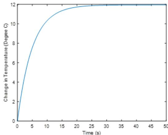
**Figure 3:** Time response of the temperature  $\Delta T(t)$  of the water.
