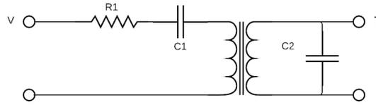
**Figure 4:** Two-port model including the iso-baric heat lost to resistor  $R_1$  in the water bath. The turns ratio of the transformer ( $a$ ) relates the voltage and current to the temperature and entropy-rate. For example  $T = V/a$  and  $\dot{S} = aI$ . Thus the units on  $a$  are either  $[V/^\circ\text{C}]$  or  $[\text{entropy-rate}/\text{A}]$ .
