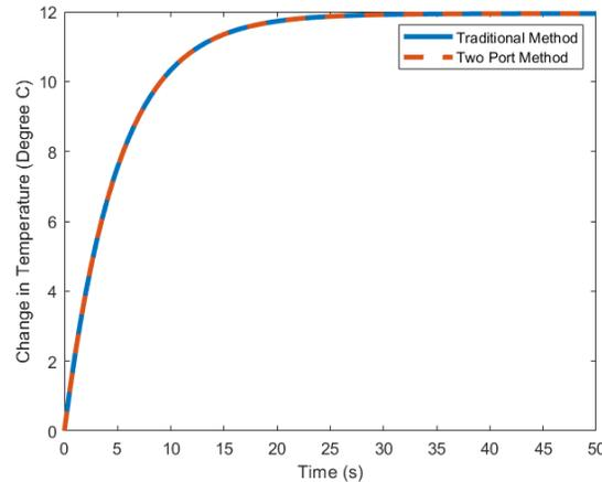
**Figure 5:** Time response of the water for both methods.
