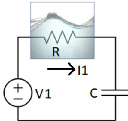
**Figure 2:** Equivalent RC circuit of Fig. 1, including the thermal losses in the resistor immersed in a water bath.
