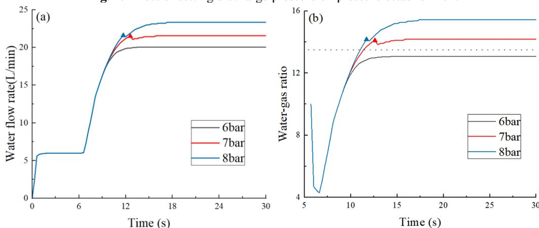
**Fig. 8.** Effect of setting discharge pressure on flow rate and water-gas ratio
