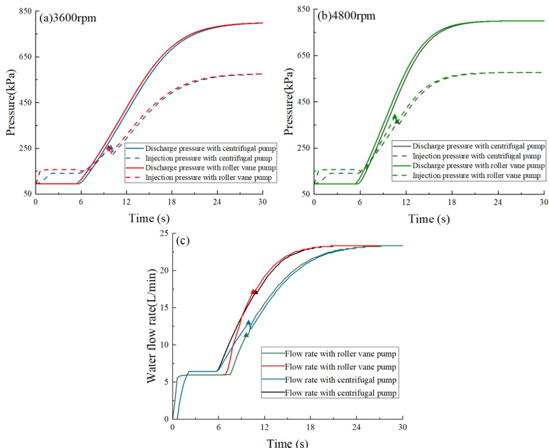
**Fig. 9.** Effect of pump type on water flow rate and pressure establishment
