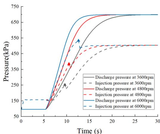
Fig. 5. Effect of rotation speed on pressure establishment
