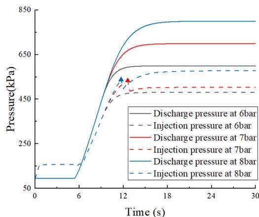
**Fig. 7.** Effect of setting discharge pressure on pressure establishment
