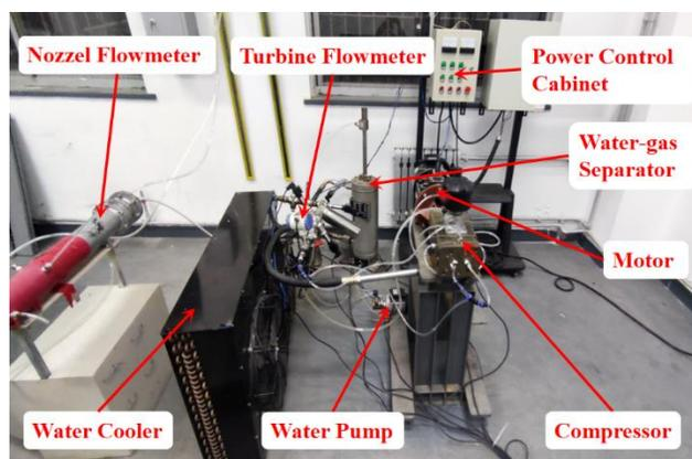
**Fig. 3.** Sketch of the experimental system components
