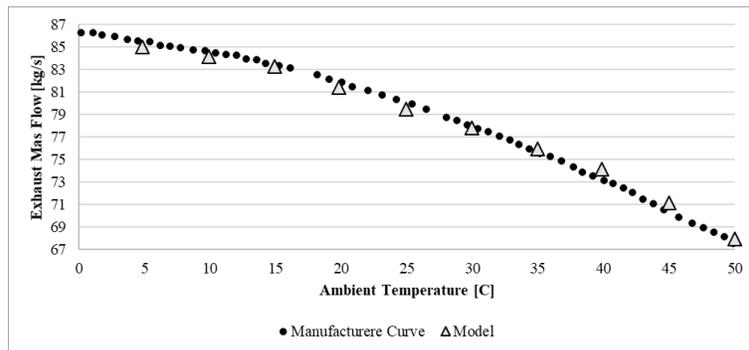
Figure 6- Exhaust Mass Flow Rate Vs. Ambient Temperature (Manufacturer curves Vs. Model result)
