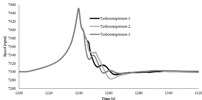
**Figure 23-**Speed profile of three compressors in the demethanizer unit for header discharge valve failure scenario (Case1)
