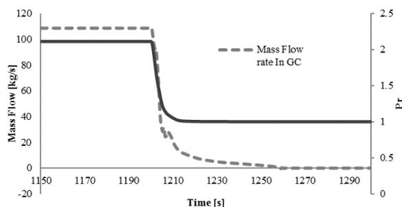
Figure11- Mass flow and pressure ratio of gas compressor for ESD Scenario (Case1)
