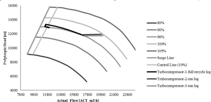
**Figure 19-**Running line of compressor for full recycle scenario (Case1)
