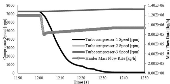
Figure13- Speed profile of turbo-compressors and header mass flow rate profile ESD scenario (Case1)
