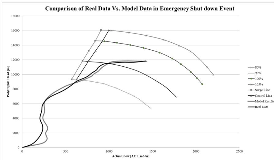
Figure 7-ESD event compressor running line (real data vs. model result)
