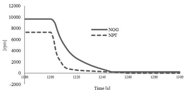
Figure12- Speed of gas generator and power turbine for ESD Scenario (Case1)
