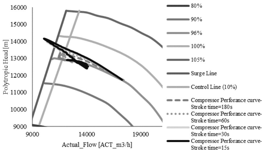
Figure 8- Stroke time sensitivity analysis during full recycle scenario
