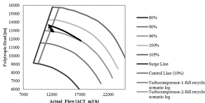
Figure 22- Running line of compressor for header discharge valve failure scenario (Case1)
