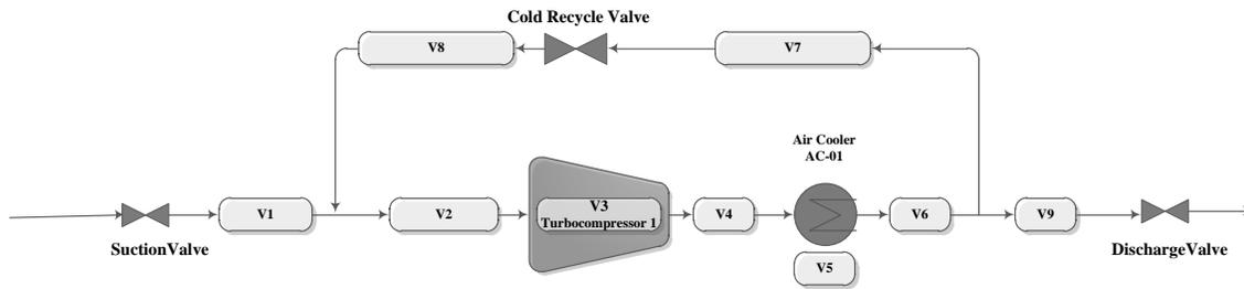
Figure 2- The 9 sub-volumes used to model single train
