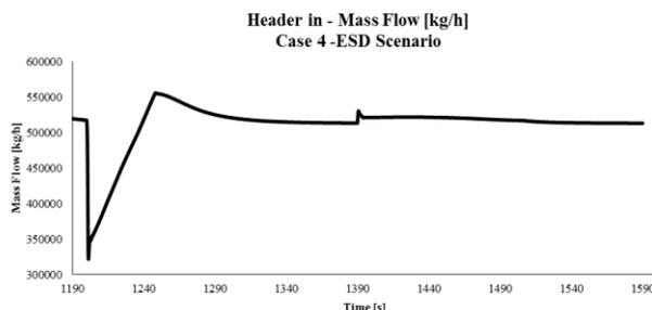
**Figure 18-** Header-suction mass flow profile for ESD scenario (Case4)
