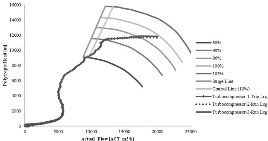
Figure 10-Running line of compressor for ESD Scenario (Case1)
