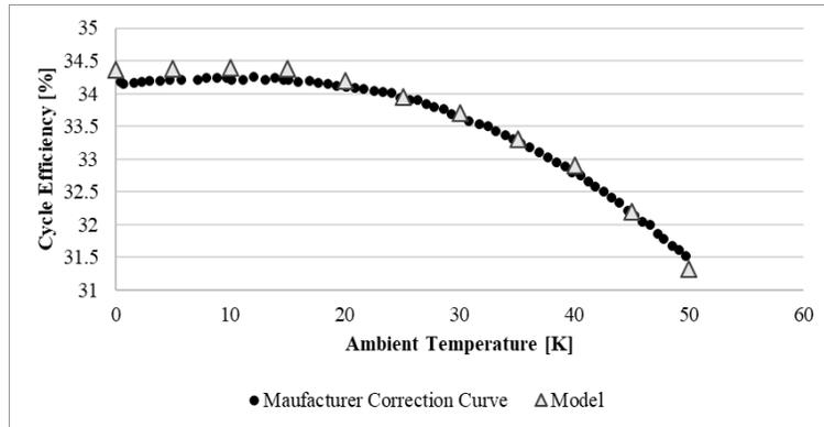
Figure 5- Turbine Efficiency Vs. Ambient Temperature (Manufacturer Curves Vs. Model result)
