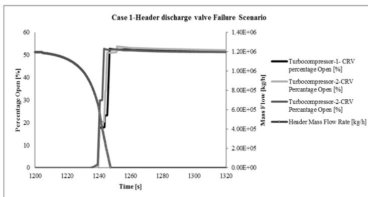
**Figure 24-**Anti-surge valves percentage open and header mass flow rate decline for header discharge valve failure scenario (Case1)
