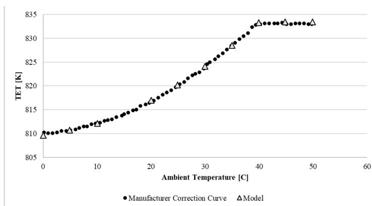
**Figure 4-** Turbine exhaust temperature Vs. Ambient temperature (Manufacturer Curves Vs. Model result)
