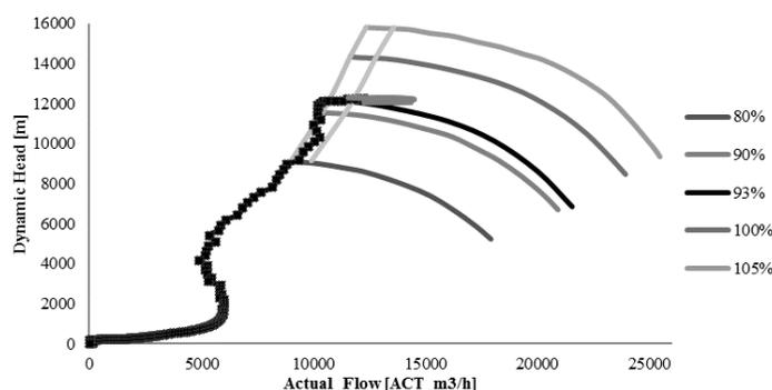
Figure 16- Running line of compressor for ESD scenario (Case 4)
