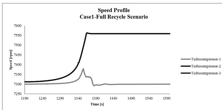
Figure 20-Speed profile of three compressors for full recycle scenario (Case1)
