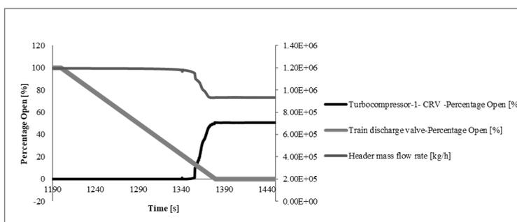
Figure 21-Header mass flow rate, anti-surge and discharge valve percentage open for full recycle scenario (Case1)
