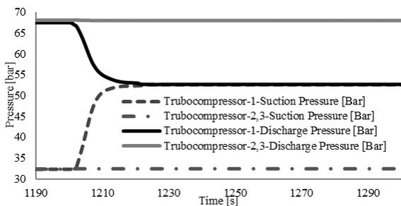
Figure14- Pressure profile of compressors in unit22 for ESD Scenario (Case1)
