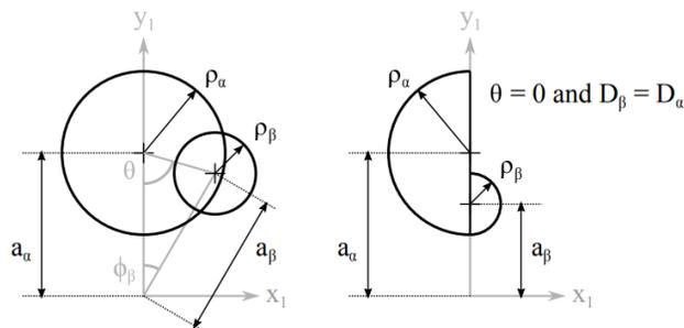
**Figure 7:** Example of the 2-pin geometry used to generate asymmetric rotor profiles; a) general case and b) simple case where  $(a_\alpha - \rho_\alpha) = (a_\beta - \rho_\beta)$ .
