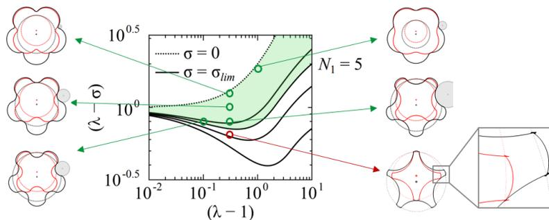
**Figure 3:** Examples of pin-generated rotor profiles with  $N_1 = 5$ . Note that undercutting can be seen on the profile that falls outside the design envelope (region shaded green)
