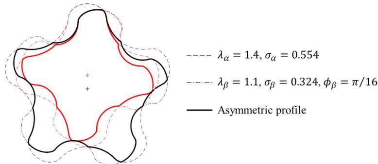
**Figure 6:** Example of general case of asymmetric rotor profile formed from pins with different values of  $a$  and  $\rho$ , but with the same value of  $E$
