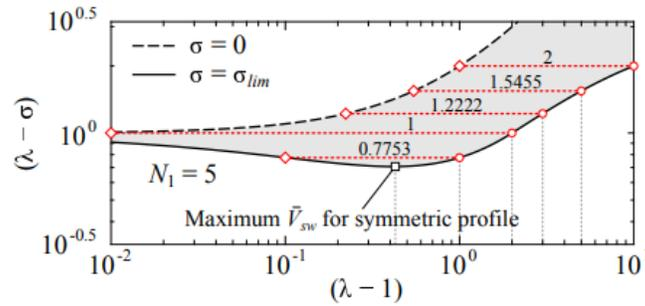
**Figure 8:** Example of the design envelope for asymmetric profiles with  $N_1 = 5$ , showing the range of possible  $\lambda$  values for constant  $(\lambda - \sigma)$  values corresponding to  $\lambda_{max} = 2, 3, 4, 6$  and  $11$ . Note that the maximum value of  $\bar{A}_{sw}$  for a symmetric profile is achieved with  $\bar{\sigma} = 1$  (i.e.  $\sigma = \sigma_{lim}$ ) and  $\lambda = 1.42$
