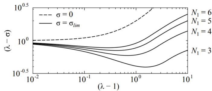
**Figure 2:** Illustration of how the maximum and minimum possible values of  $\sigma$  as a function of  $N_1$  and  $\lambda$  allow the design envelope of symmetric rotor profiles to be defined.
