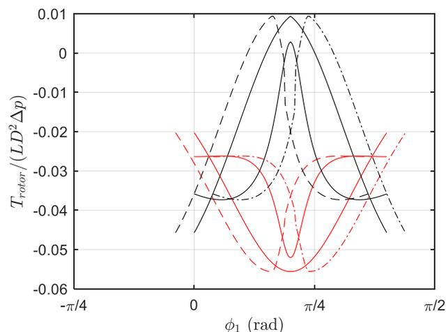
**Figure 12:** Influence of rotor profile on the net rotor torque for the symmetric (solid lines) and asymmetric (dashed lines) profiles shown in Figure 11
