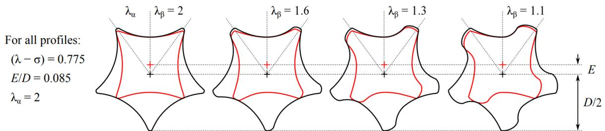
**Figure 9:** Examples of asymmetric pin-generated rotor profiles with  $N_1 = 5$  and  $(\lambda - \sigma) = 0.775$ . All profiles are shown with the same value of  $D$
