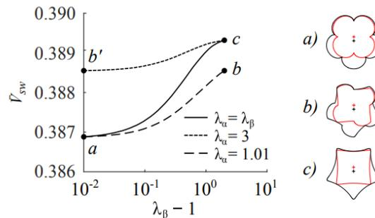
**Figure 10:** Normalised swept area for symmetric and asymmetric rotor profiles as function of  $\lambda$  for  $(\lambda - \sigma) = 1$  and  $N_1 = 5$ . Note that the profile for point  $b'$  is the mirror image of  $b$ .
