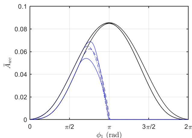
**Figure 11:** Working chamber area (black lines) and inlet port area (blue lines) for symmetric (solid lines;  $\lambda = 1.1$ ,  $\lambda = 2$ ) and asymmetric (dashed lines;  $\lambda_\alpha = 1.1$  &  $\lambda_\beta = 2$ , and vice versa) rotor profiles with  $N_1 = 5$  and  $(\lambda - \sigma) = 0.775$
