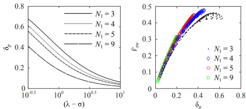
**Figure 5:** Relative profile depth for the outer rotor as a function of  $N_1$  and  $(\lambda - \sigma)$ , and the influence on swept area per revolution of the inner rotor,  $\bar{A}_{sw}$
