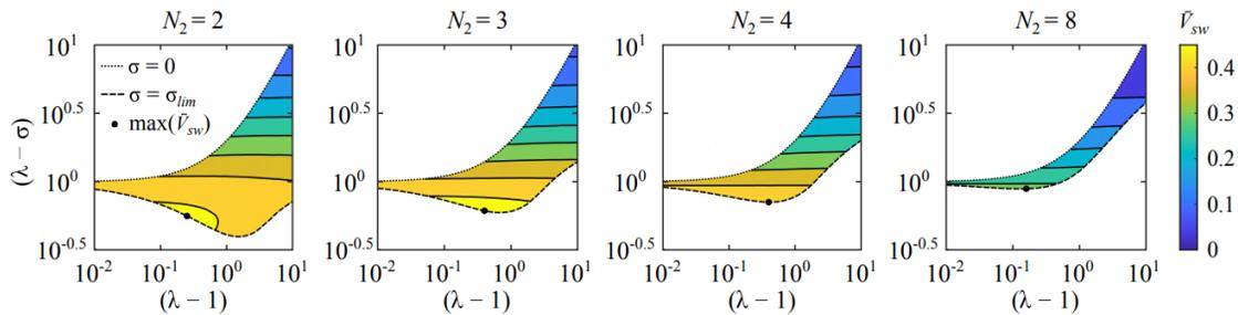
**Figure 4:** Normalised swept area per revolution of inner rotor for symmetric rotor profiles as function of  $\lambda$  and  $(\lambda - \sigma)$  for specified values of  $N_1$
