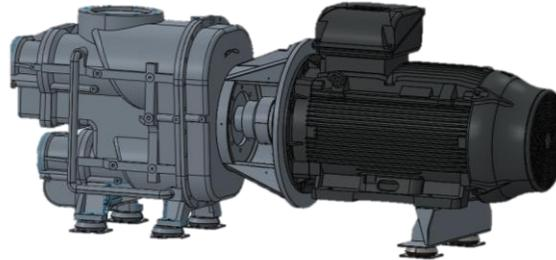
**Figure 1.** General view of the double-stage screw compressor
