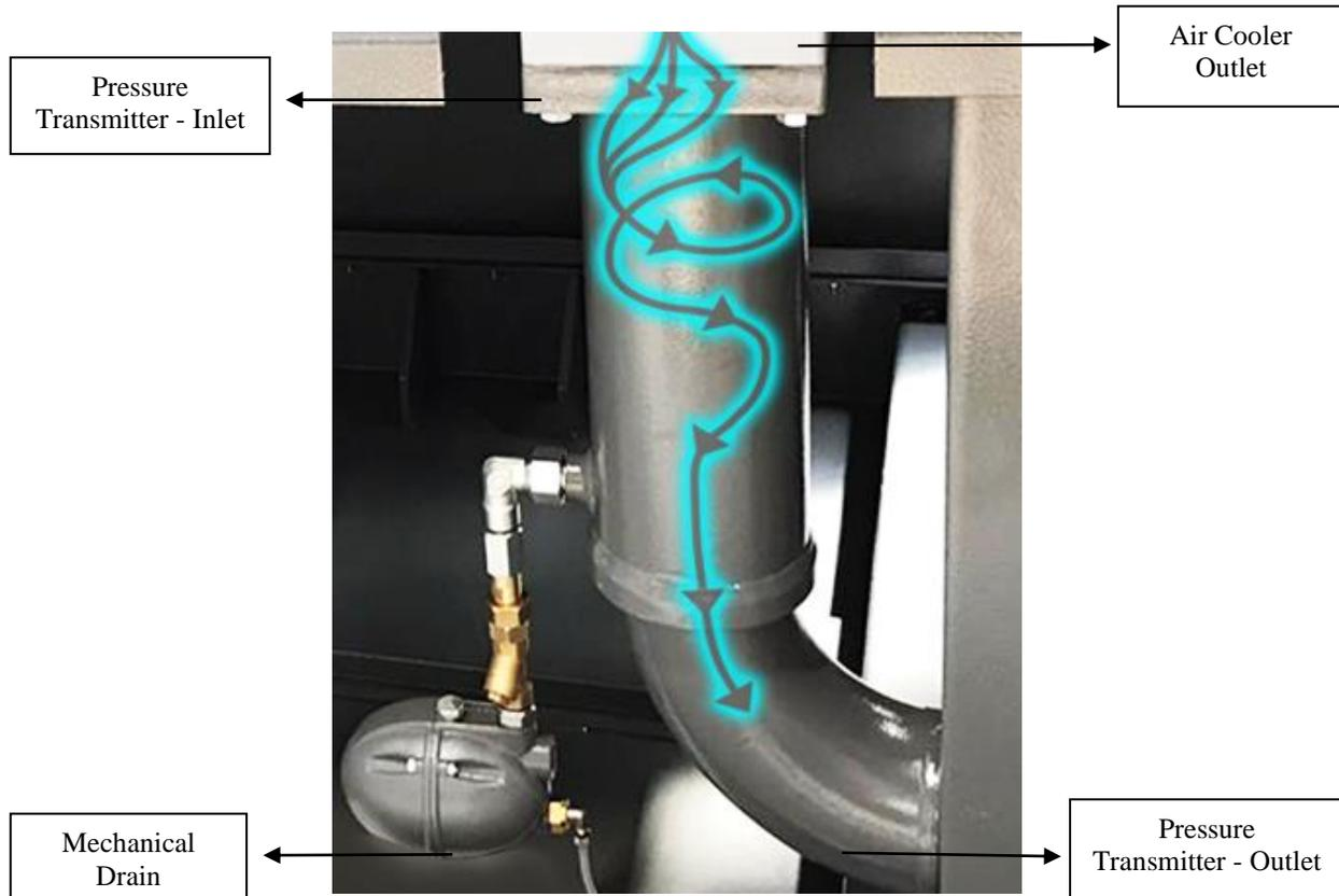
**Figure 4:** Water (Condense) Separator
