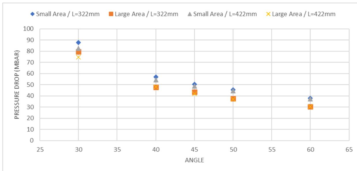
**Figure 6:** Condense Separator Dimensions vs Pressure Drop (pa)
