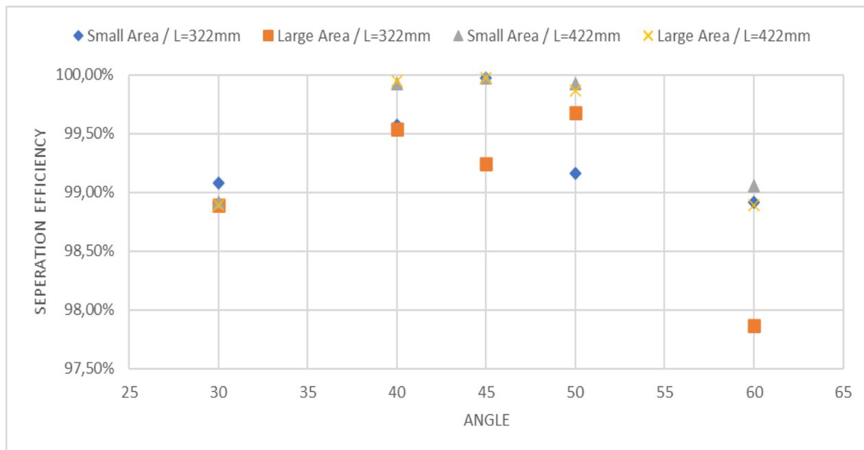
**Figure 5:** Condense Separator Dimensions vs Separation Efficiency (%)
