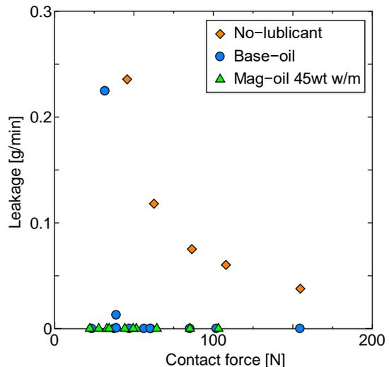
**Figure 11:** Relationship between contact force and gas leakage at 0.4 MPa.
