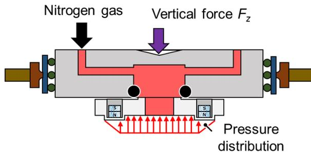
**Figure 8:** Conceptual model of the pressure distribution for calculation of pressure force.
