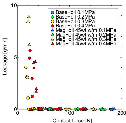
**Figure 12:** Relationship between contact force and gas leakage by friction and leakage simultaneous test.
