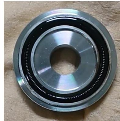
Figure 4: Application of magnetic nano-oil to the test piece.
