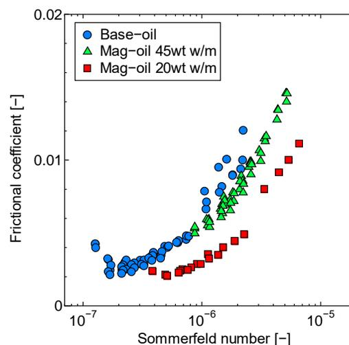
**Figure 7:** Stribeck curve for friction single test.
