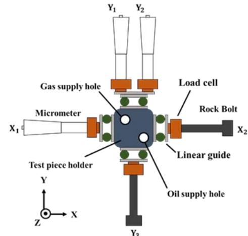
Figure 2: Detailed diagram of the test piece holder.
