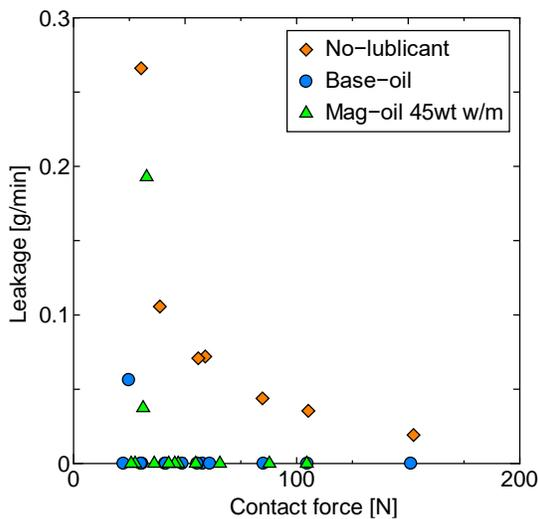
**Figure 10:** Relationship between contact force and gas leakage at 0.3 MPa.
