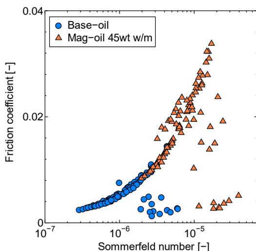
**Figure 14:** Stribeck curve by friction and leakage simultaneous test.
