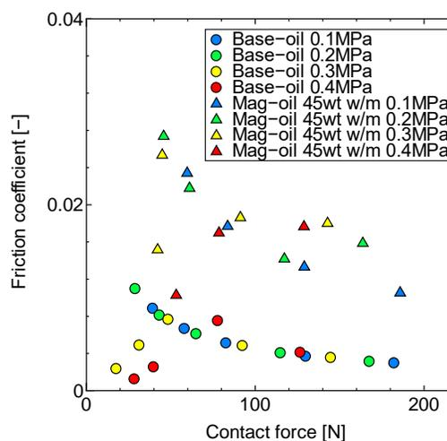
**Figure 13:** Relationship contact force and friction coefficient at 300 rpm by friction and leakage simultaneous test.
