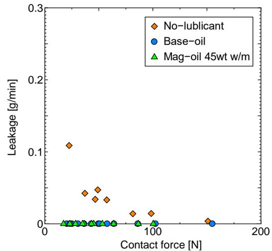
**Figure 9:** Relationship between contact force and gas leakage at 0.2 MPa.
