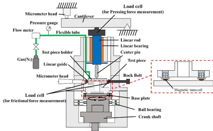
Figure 1: Experimental apparatus.
