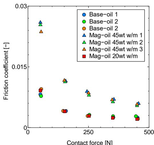
**Figure 6:** Relationship between contact force and friction coefficient at 300 rpm.
