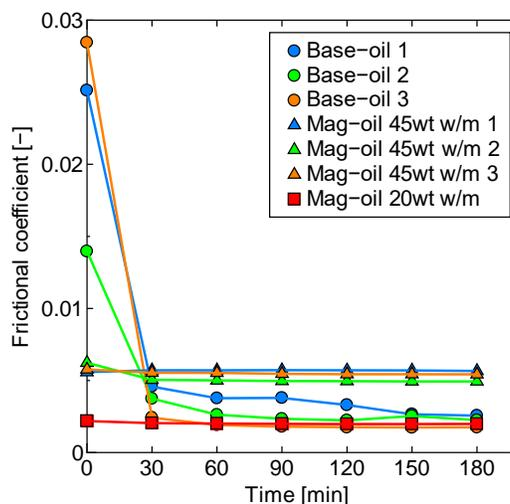
**Figure 5:** Time series difference of the frictional coefficient for the pre-conditioning interim operation.
