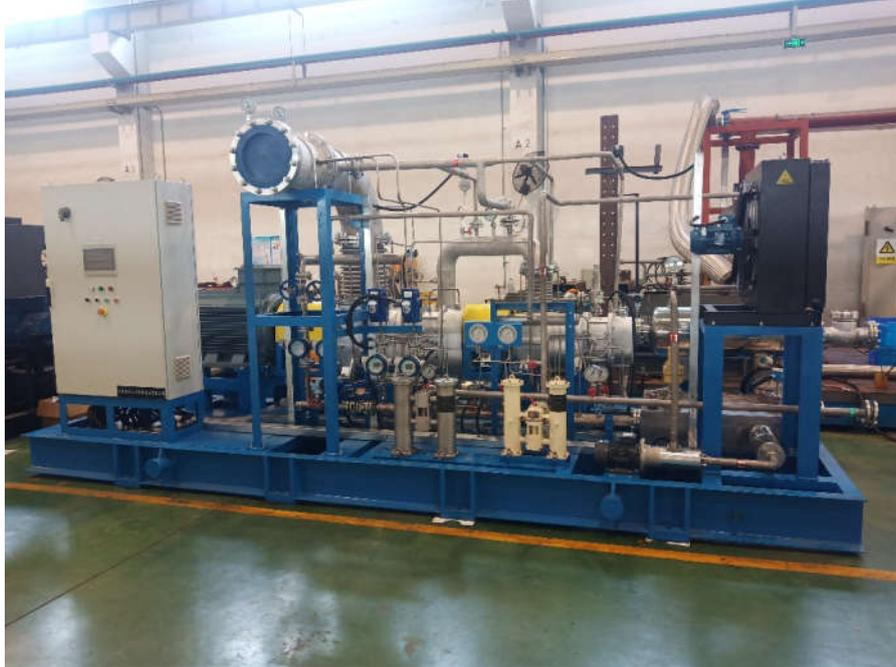
**Figure 4:** Picture of the developed twin-screw steam compressor
