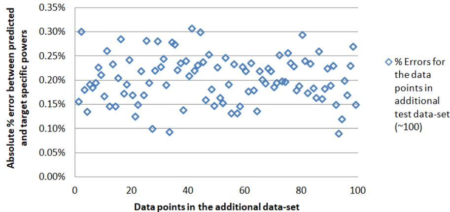
**Figure 6:** Absolute %errors between specific powers predicted by NN and those calculated by solving the chamber model for all the profiles in the additional testing data-set
