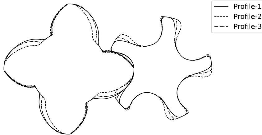
**Figure 1:** Three retrofitted 4/5 N-rotor profiles with different set of profile input parameters ( $R_1$ ,  $R_2$ ,  $R_3$ ,  $R_4$  &  $n$ )
