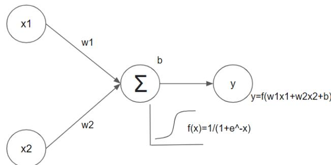
**Figure 4:** Working of a neuron in an artificial neural network with two inputs and single output
