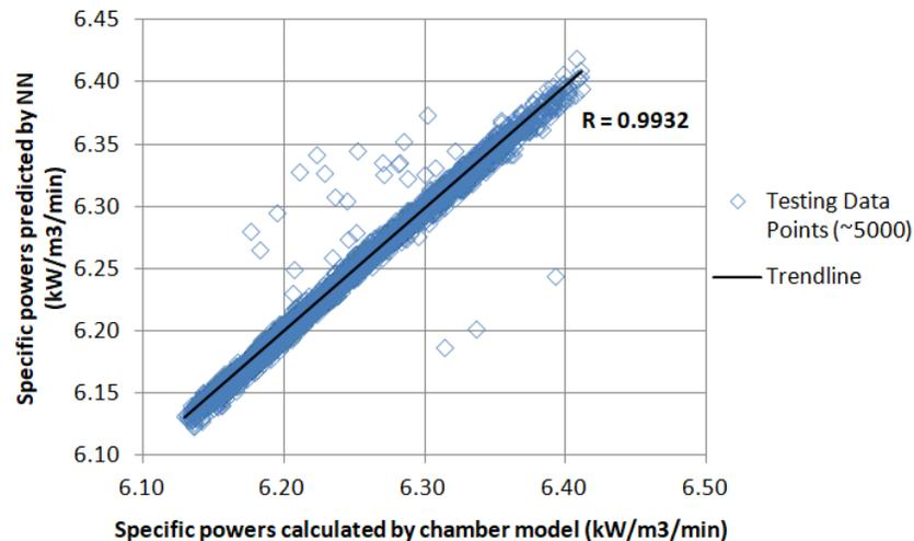
**Figure 5:** Plot of the specific powers predicted by NN against those calculated by solving the chamber model for all the profiles in testing data-set
