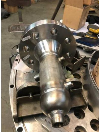
**Figure 1: Fabricated compression chamber**
