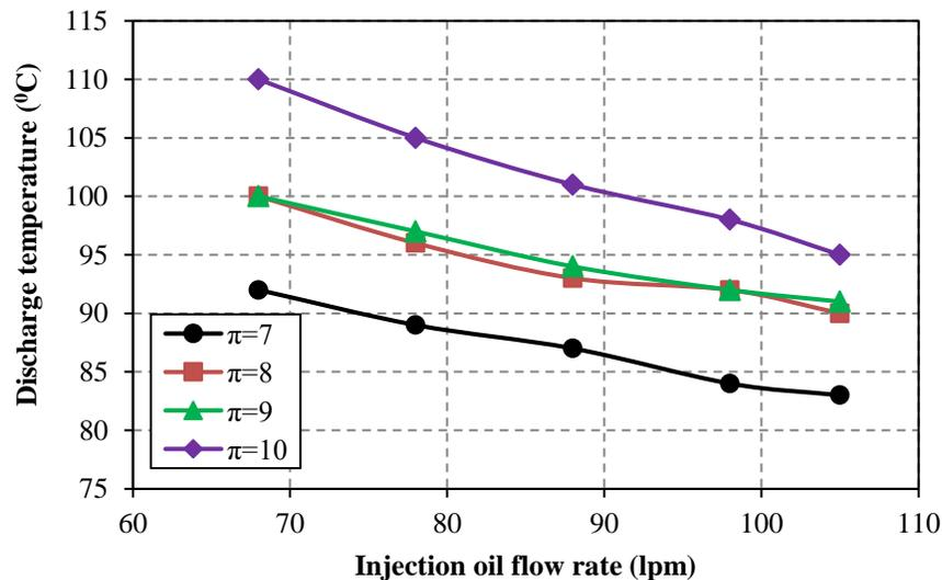
**Figure 4.** Discharge temperature at different pressure ratios vs. oil flow rate
