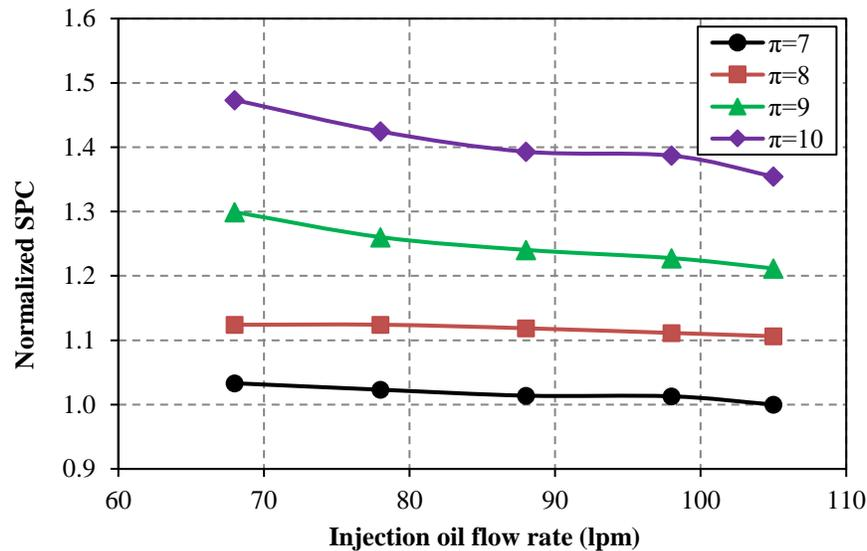
**Figure 3.** Normalized SPC at different pressure ratios vs. oil flow rate
