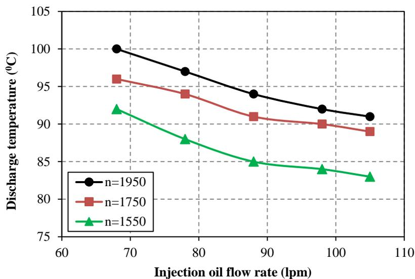
**Figure 7.** Discharge temperature at different pressure ratios vs. oil flow rate
