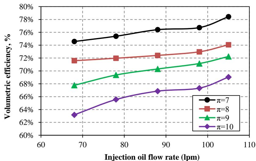
Figure 2. Volumetric efficiency at different pressure ratios vs. oil flow rate
