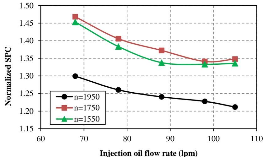
**Figure 6.** Normalized SPC at different speed vs. oil flow rate
