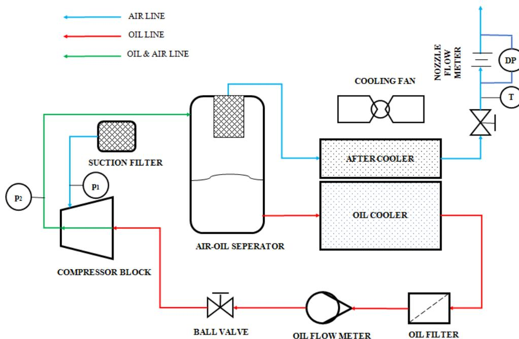
**Figure 1.** Schematic of the flow diagram
