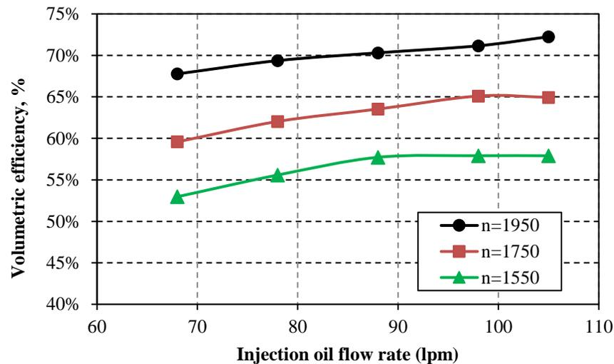
**Figure 5.** Volumetric efficiency at different speeds vs. oil flow rate
