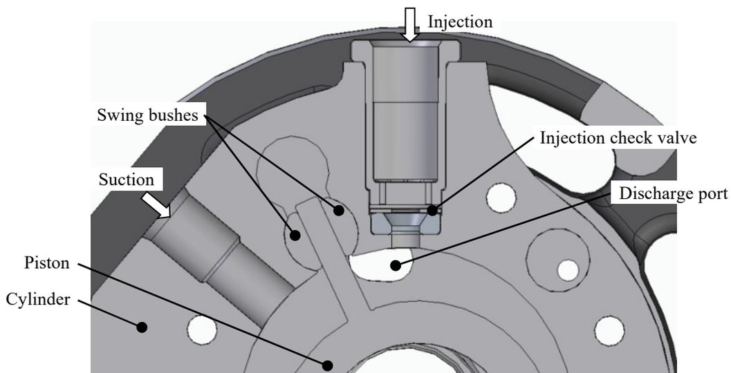
**Figure 5:** Details of side port injection mechanism
