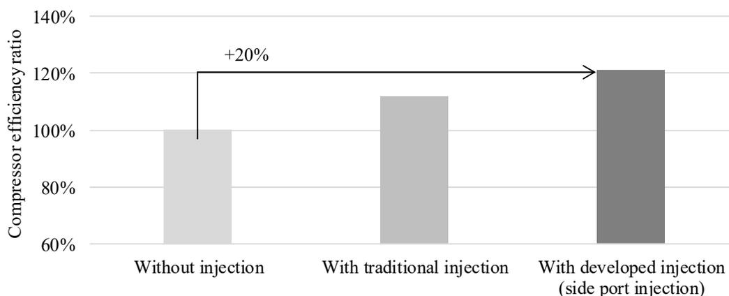
**Figure 10:** Efficiency ratio between with/without injection
