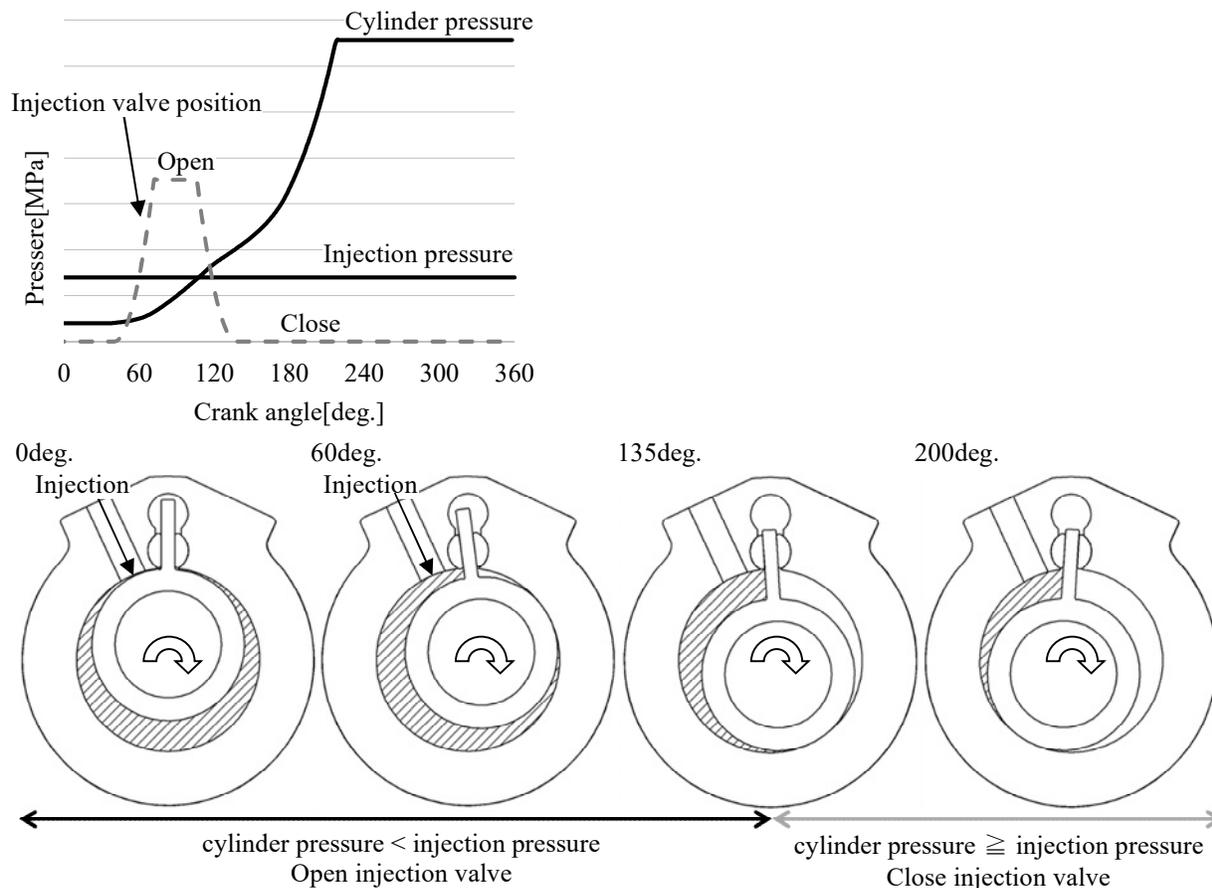
**Figure 6:** Relation between opening and closing of injection valve and cylinder pressure during one rotation
