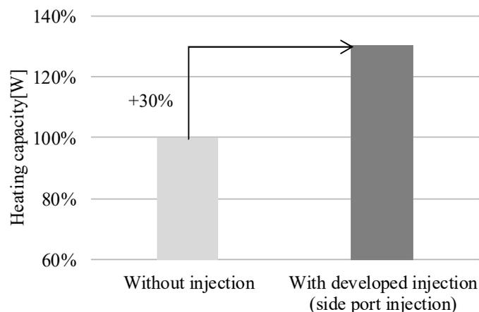
**Figure 8:** Heating capacity between with/without injection
