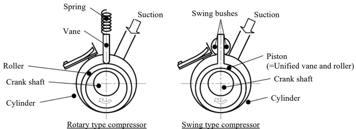
**Figure 3:** Mechanism of Rotary and Swing type compressor
