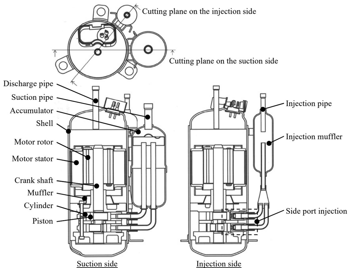
**Figure 4:** Cross sectional view of Swing type Compressor with side port injection
