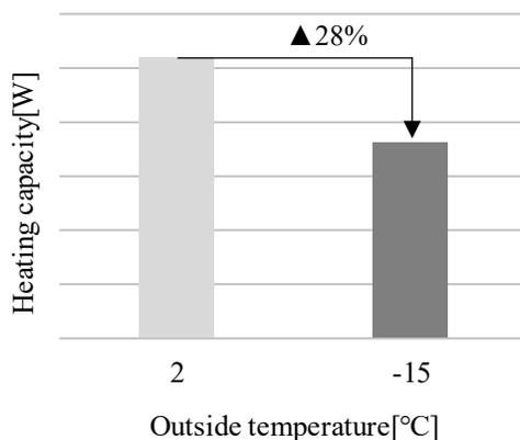
**Figure 1:** Relationship between heating capacity and outside temperature
