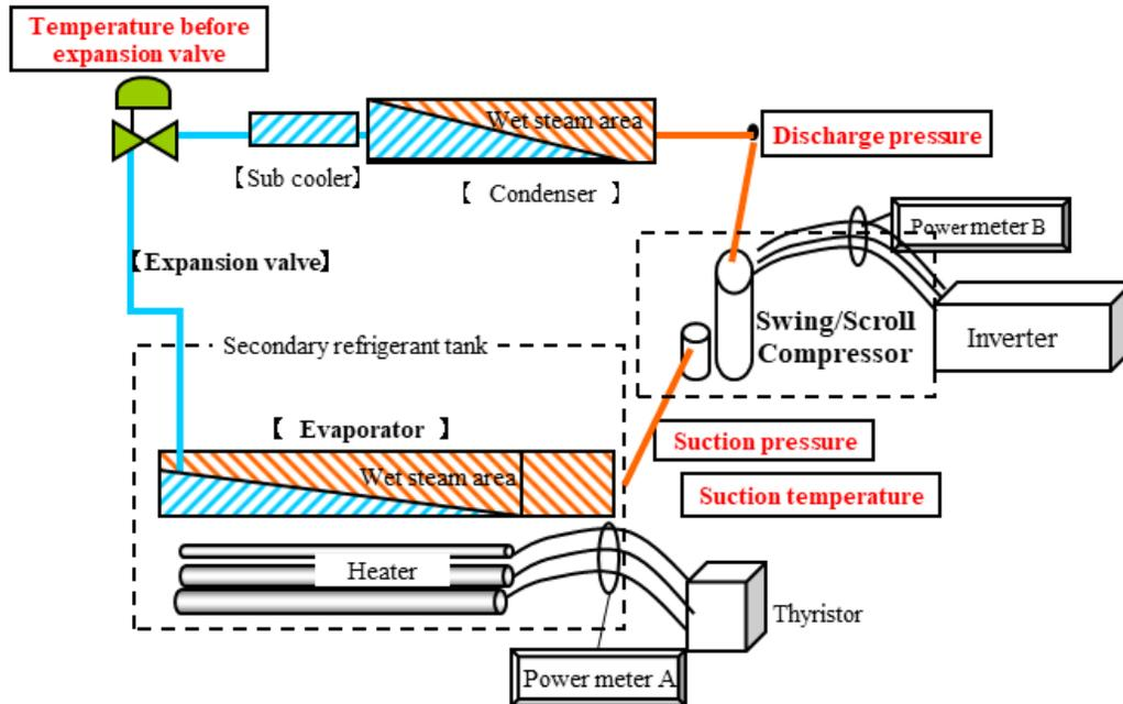
Figure 2: Test equipment: Calorimeter
