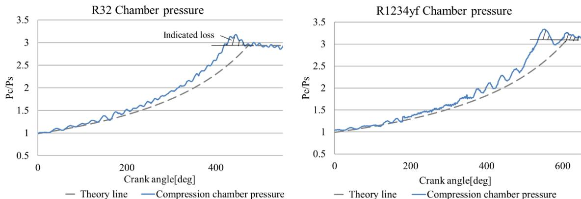
**Figure 5:** Internal pressure diagram of scroll compressor
