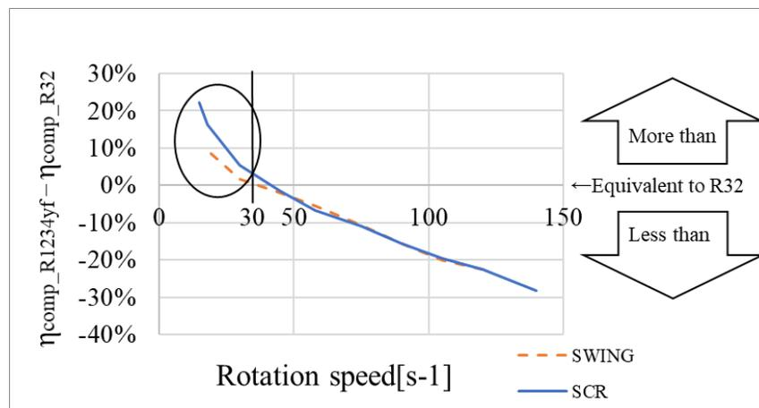
Figure 3: Compressor efficiency for R32 refrigerant
