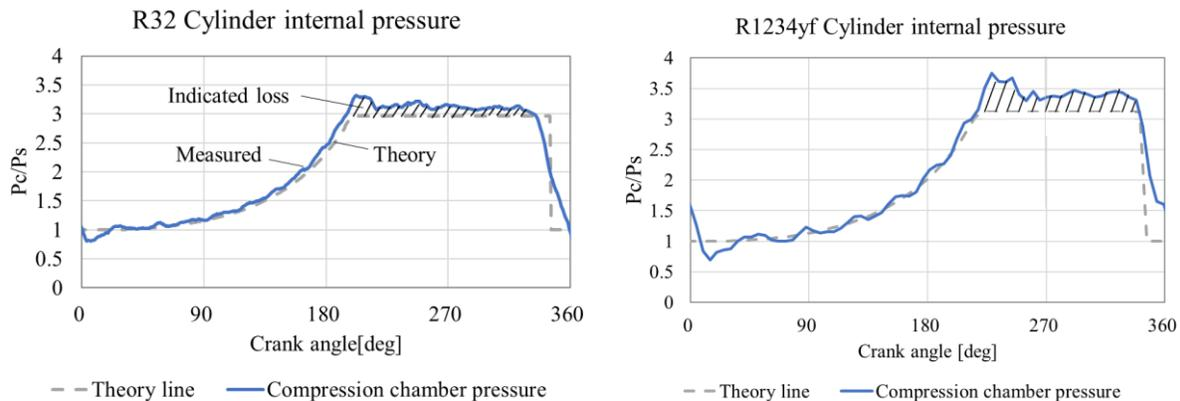
**Figure 4:** Internal pressure diagram of swing compressor
