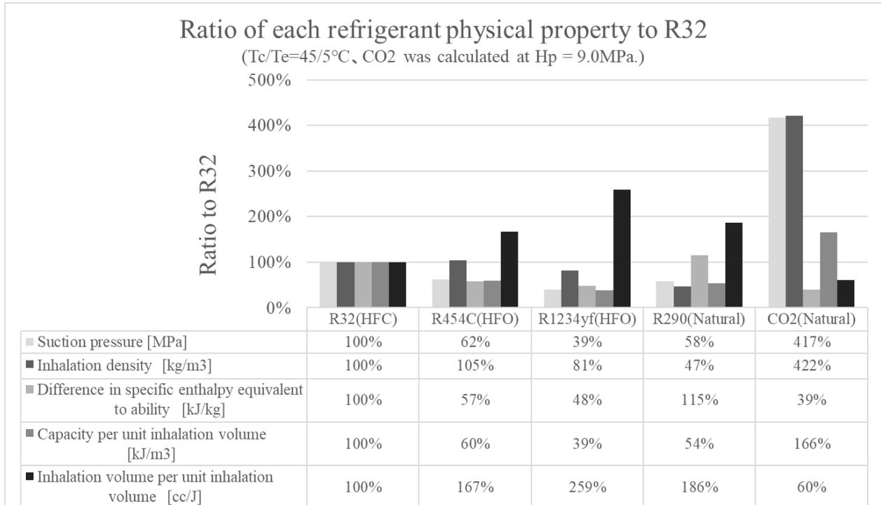
**Figure 1:** Ratio of each refrigerant physical property to R32
