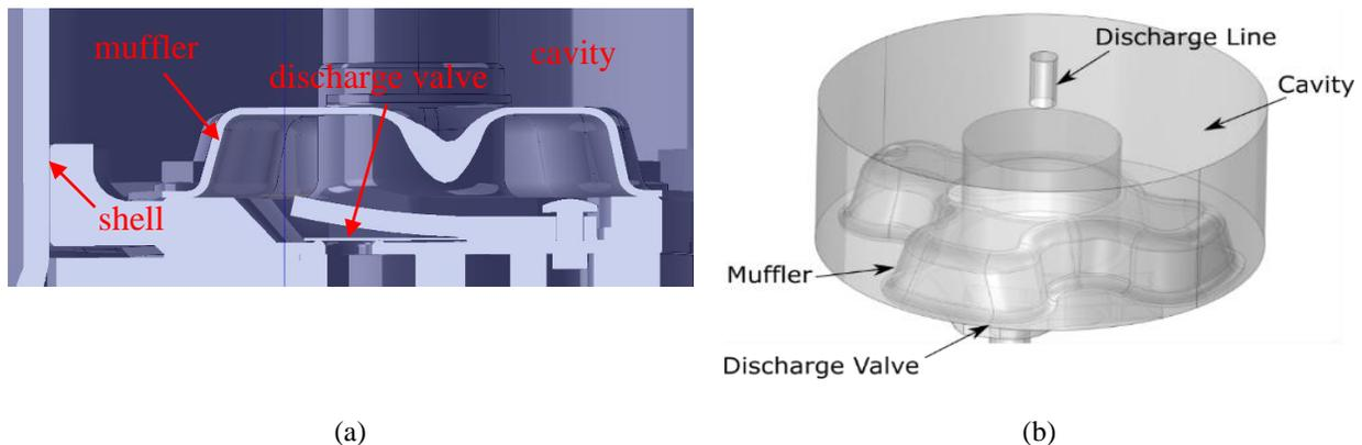
**Figure 4:** (a): Vicinity of compressor discharge port; (b): Compact CFD simulation domain
