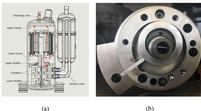
**Figure 1:** (a) typical structure of a rolling piston compressor; (b) compression chamber of a rolling piston compressor
