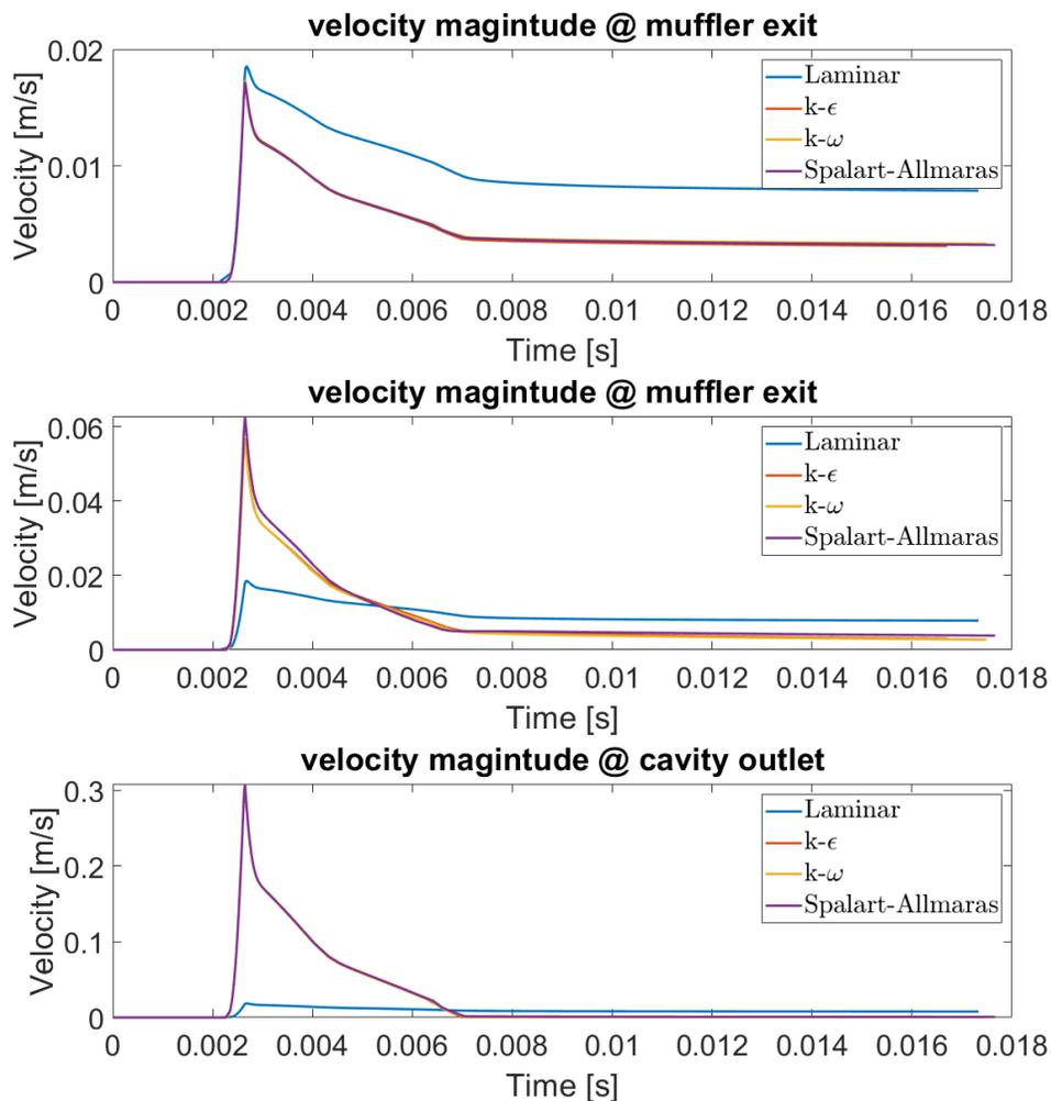
**Figure 7.** Effect of turbulence model on fluid field solution
