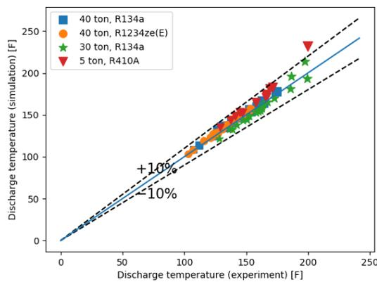
**Figure 3:** Discharge temperature for various refrigerants and displacement volumes. Marker size is proportional to the experimental uncertainty.
