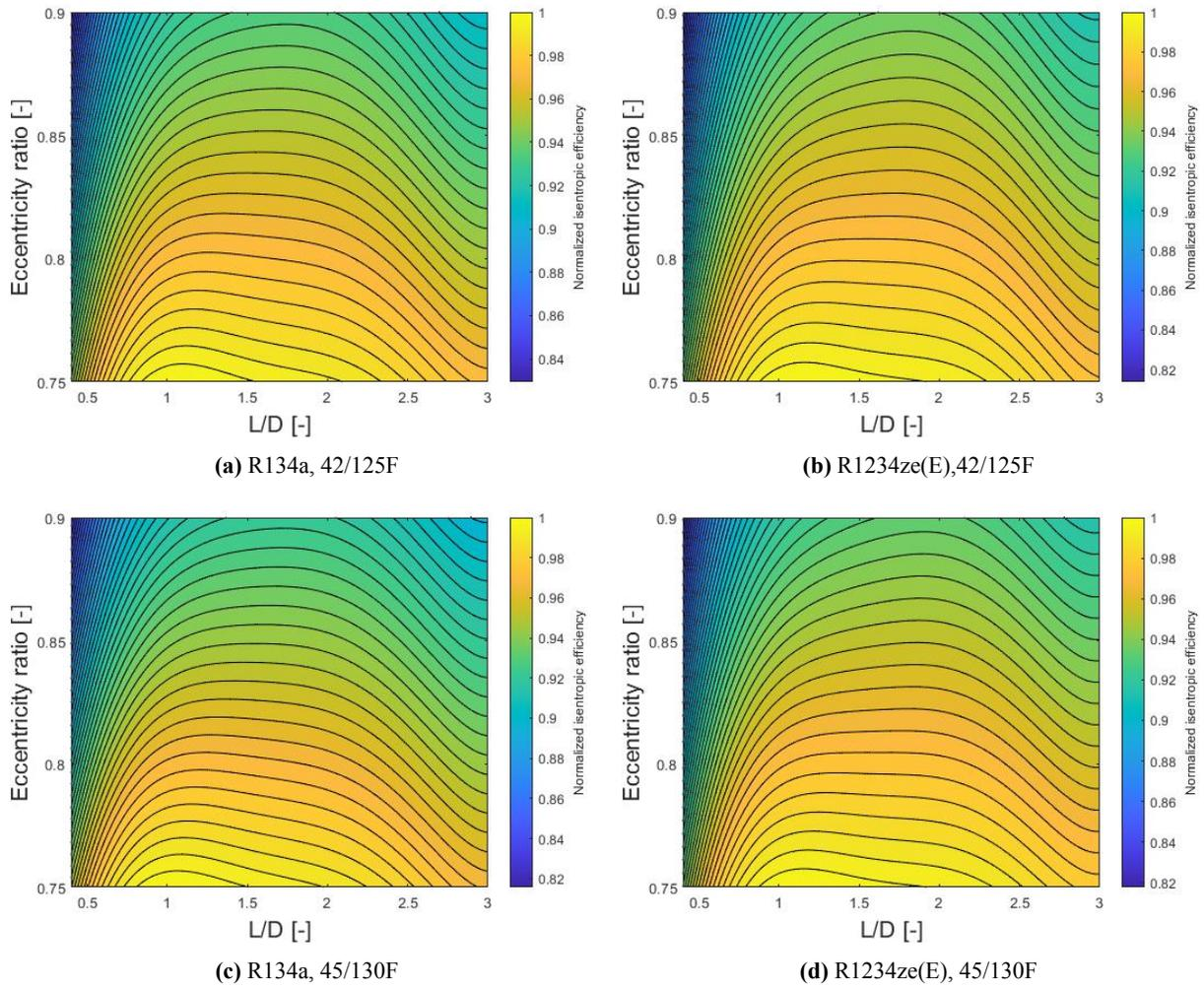
**Figure 4:** Isentropic efficiency for different refrigerants and operating conditions.
