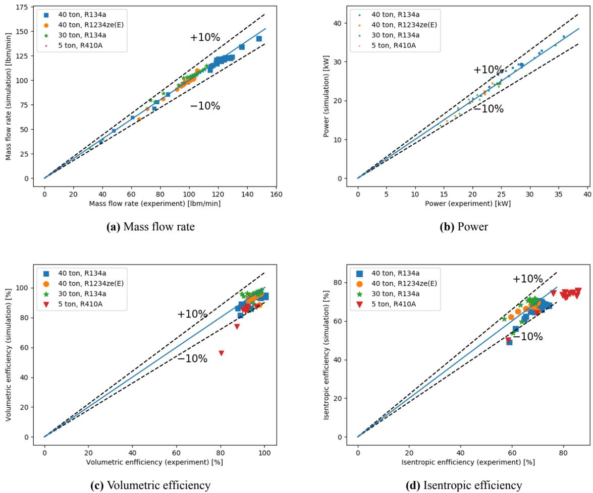
**Figure 2:** Model validation using various refrigerants and displacement volumes. Marker size is proportional to the experimental uncertainty.
