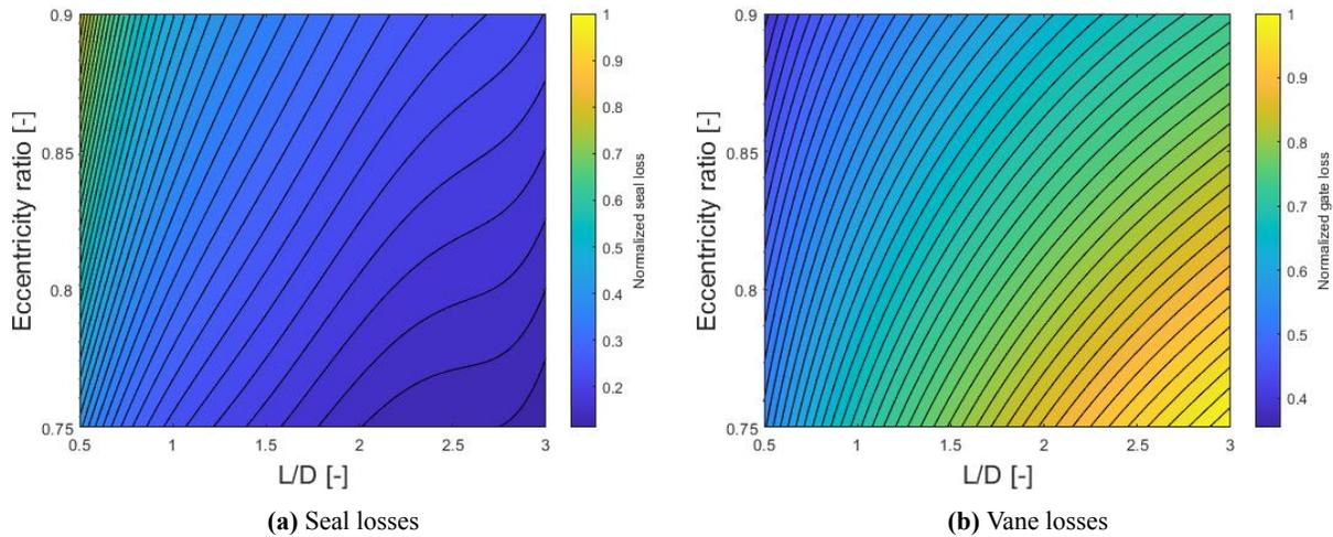
**Figure 6:** Mechanical losses in spool compressor for R134a various aspect ratio at 45/130F condition.
