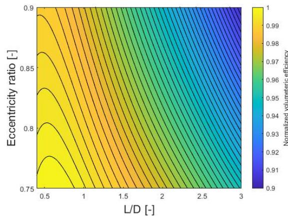
**Figure 5:** Volumetric efficiency for R134a at 45/130F.
