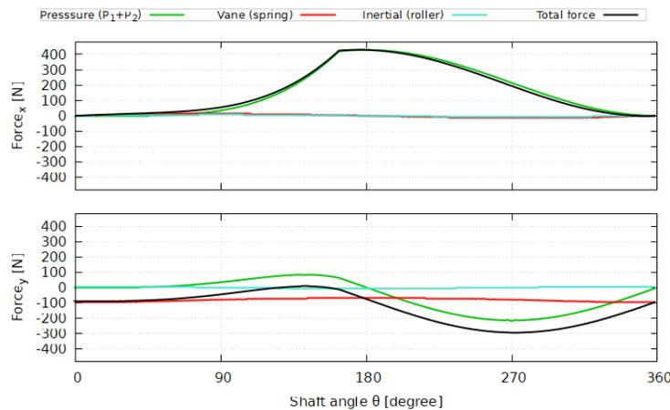
**Figure 7:** Acting forces on the roller as a function of the rotation angle
