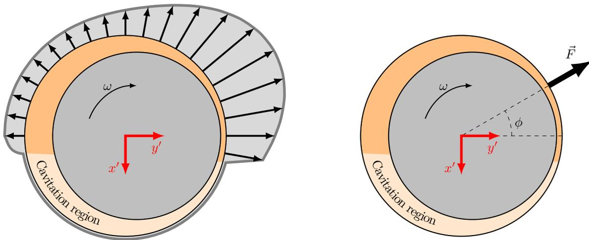
**Figure 4:** Pressure distribution (left) and global force and angle with respect to  $h_{min}$  (right)
