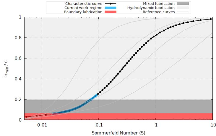
**Figure 8:** Lubrication regime  $\Lambda$  for the Roller-Cam interface
