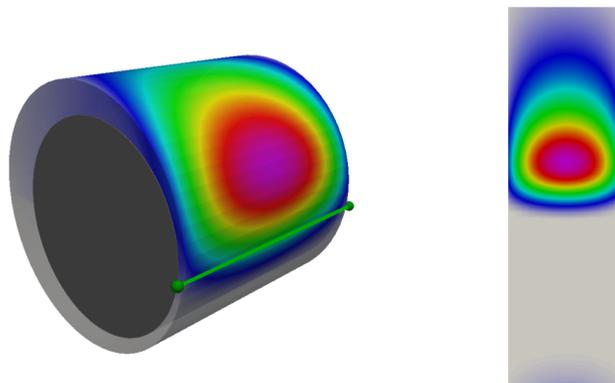
**Figure 5:** Pressure distribution field for a bearing. The line indicates the minimum film thickness position.
