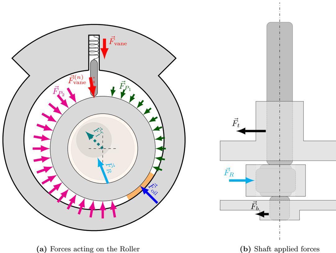
**Figure 6:** Acting forces on the rotary compressor
