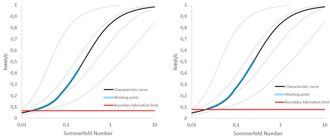
**Figure 10:** Change of working regime from thermal expansion between room temperature (left) and surfaces at 100 °C (right) keeping the rest of variables constant.
