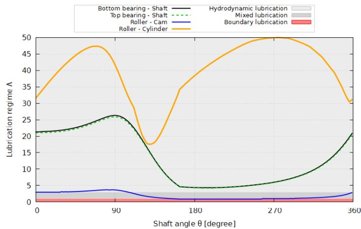
**Figure 9:** Lubrication regime  $\Lambda$  for the Roller-Cam interface
