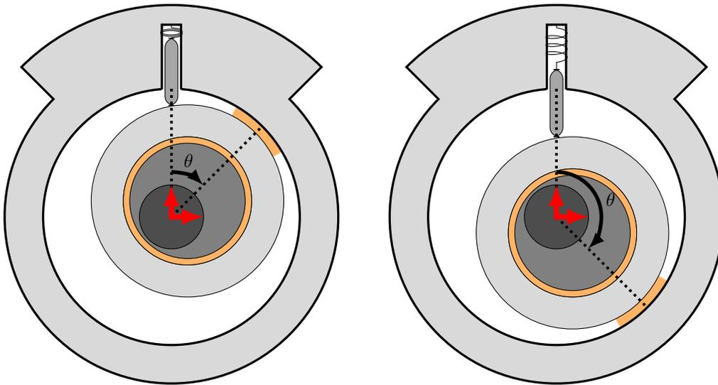
**Figure 3:** Shaft angle  $\theta$  definition
