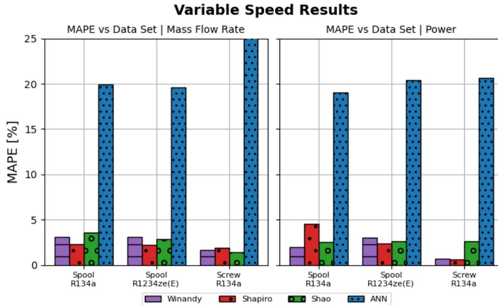
**Figure 4:** Mass flow rate and power results under modulation (variable speed) testing
