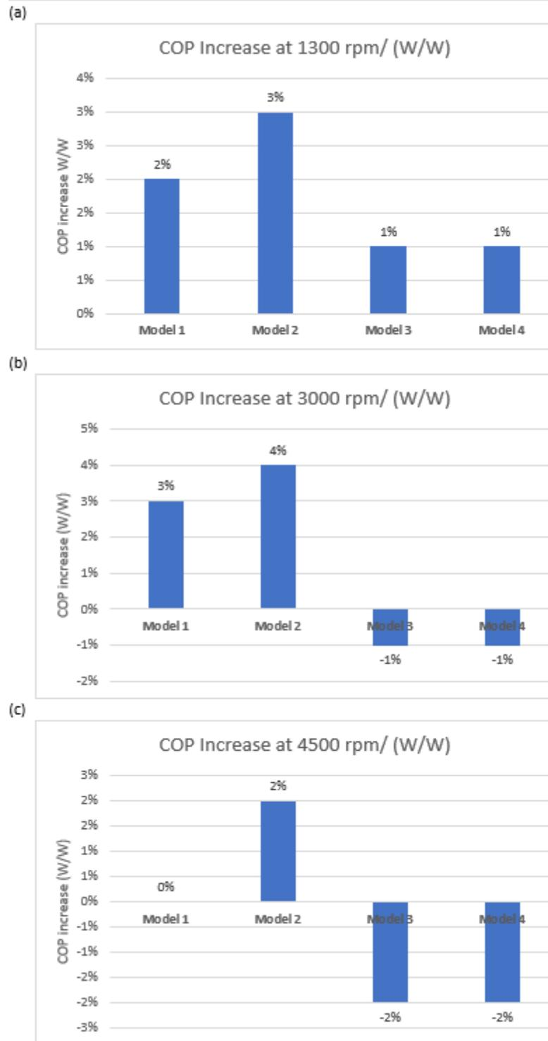
**Figure 3:** (a) Change in COP at 1300 rpm (b) Change in COP at 3000 rpm (c) Change in COP at 4500 rpm
