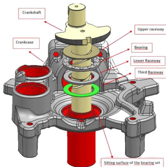
**Figure 1: Schematic of the bearing set**
