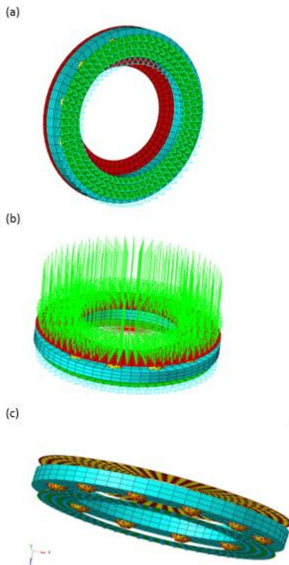
**Figure 2:** (a) Fixed constraint on the lower raceway (b) 10 bar pressure on the upper raceway (c) Freeze contact.
