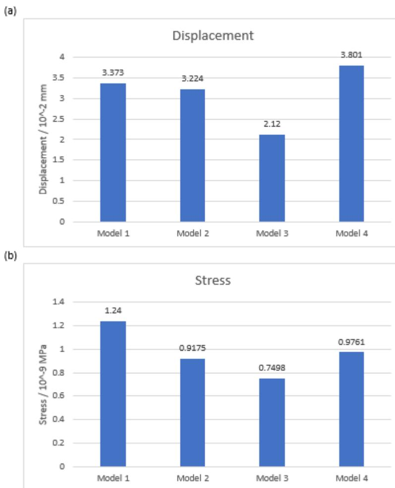
**Figure 4:** (a) Displacement of the balls of the compressor (b) Stress on the balls of the compressor
