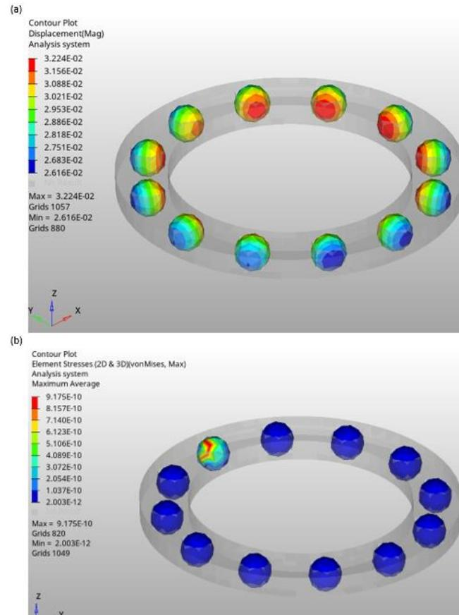
**Figure 5:** (a) Displacement on the balls of the bearings (b) Stress on the balls of the bearings
