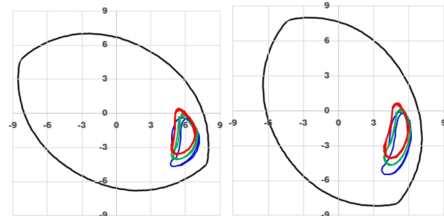
Figure 8c: Trajectories of Lobe bearing( \Phi=120^\circ, 150^\circ )
