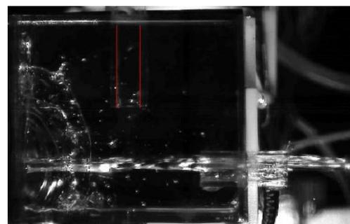
(g) Oil dispersion inside the muffler (Test 4).
