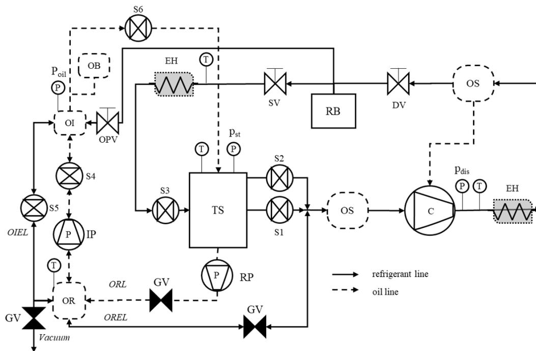
Figure 3: Overall representation of the test section.
