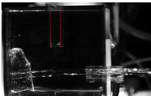
(e) Oil dispersion inside the muffler (Test 1).
