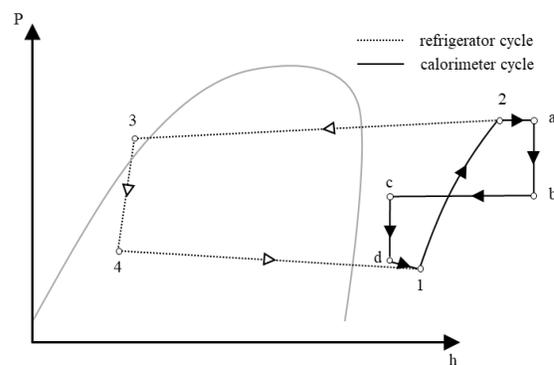
Figure 2: p-h diagram associated with the hot-cycle calorimeter and refrigeration cycle.
