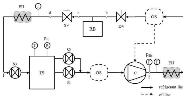
Figure 1: Schematic of the test bench.
