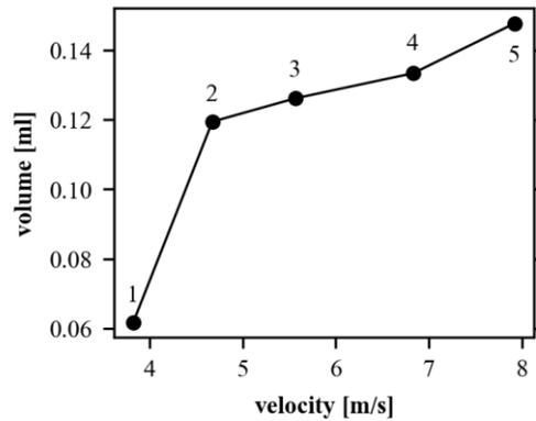
**Figure 6:** Collected volume of oil as a function of the injection velocity.
