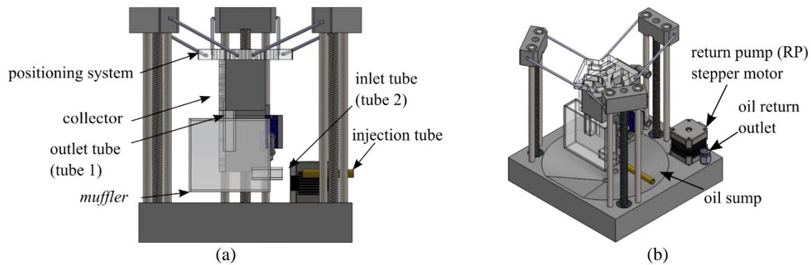
**Figure 5:** Test section. (a) front view; (b) isometric view.
