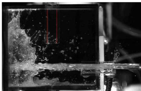
(h) Oil dispersion inside the muffler (Test 6).
