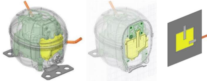
**Figure 4:** Simplified suction muffler geometry (Rodrigues, 2018).
