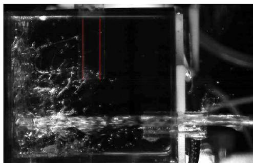
(f) Oil dispersion inside the muffler (Test 5).
