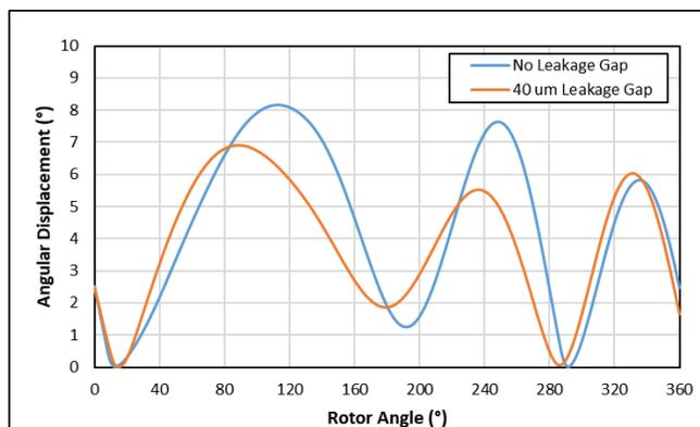
**Figure 15:** Reed valve opening over a period of cycle
