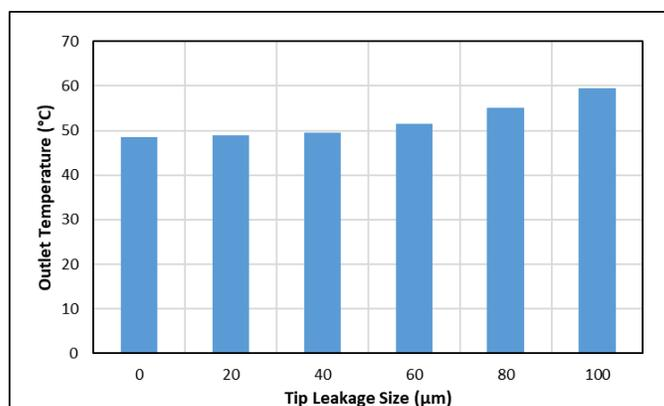
**Figure 8:** Temperature at outlet boundary of E-compressor for different tip leakage sizes
