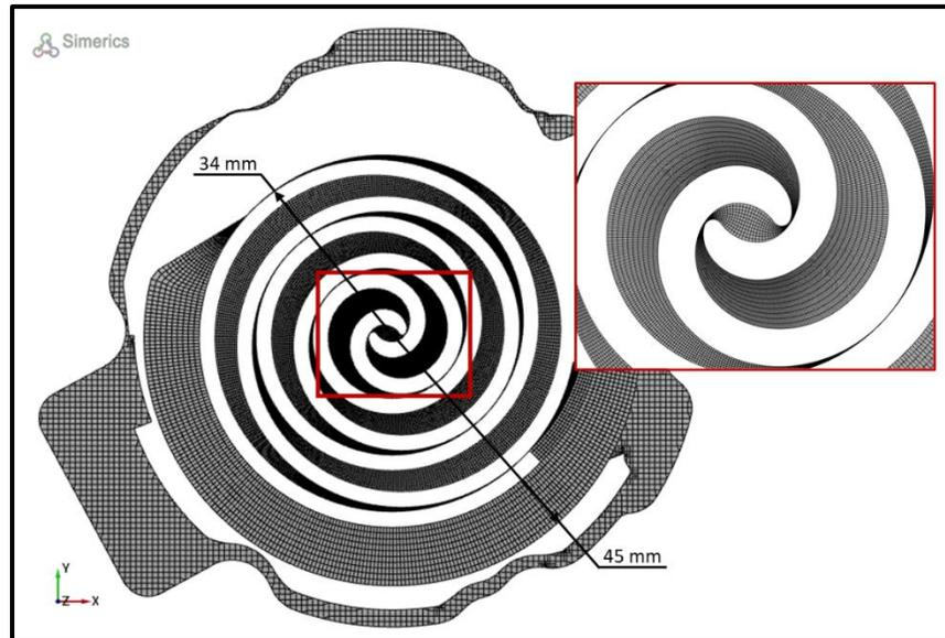
**Figure 1:** Cross-section view of scroll rotor template mesh.
