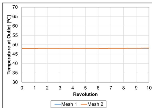
**Figure 4:** Comparison of temperature at outlet boundary between cases with different mesh settings.
