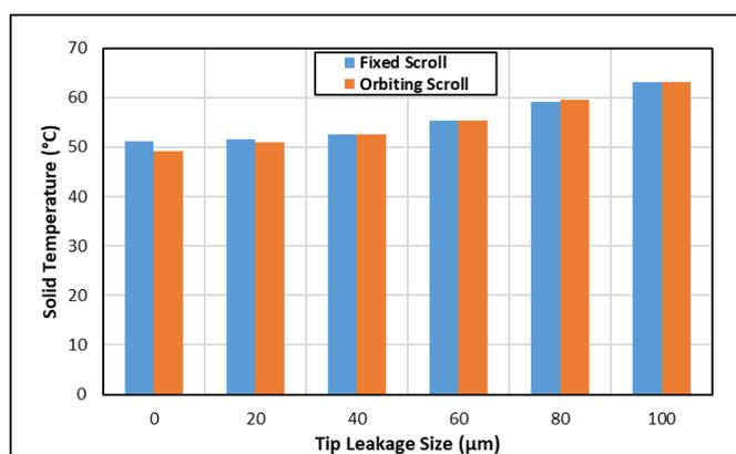
**Figure 10:** Maximum Solid Temperature in scroll solids for different tip leakage sizes
