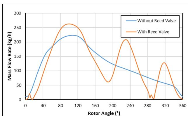
**Figure 14:** Outlet mass flow rate at discharge port of scroll compressor for Case 1
