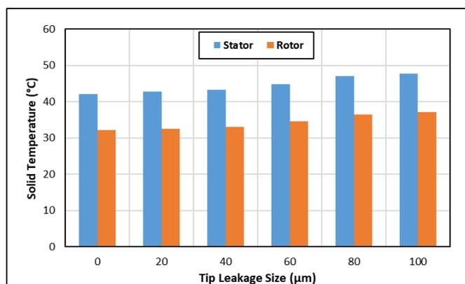
**Figure 9:** Maximum Solid Temperature in motor solids for different tip leakage sizes
