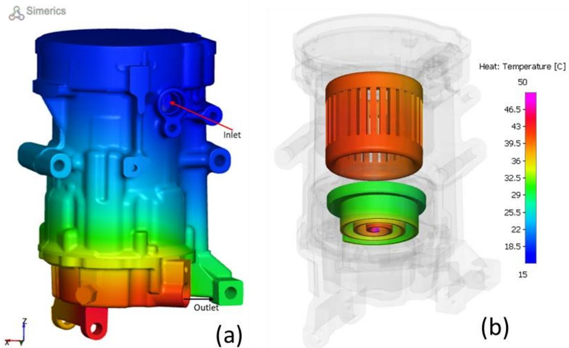
**Figure 12:** Temperature contours on the E-compressor (a) casing, (b) coil and orbiting scroll for Case 1
