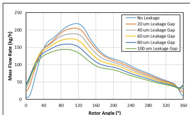
**Figure 6:** Outlet mass flow rate at discharge port of scroll compressor.
