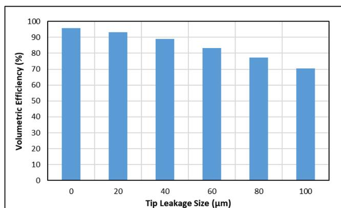
**Figure 7:** Volumetric Efficiency for different tip leakage sizes
