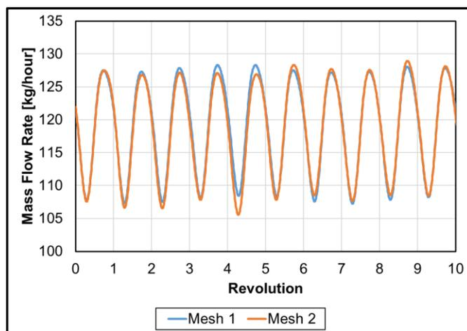
**Figure 3:** Comparison of mass flow rate through outlet boundary between cases with different mesh settings.
