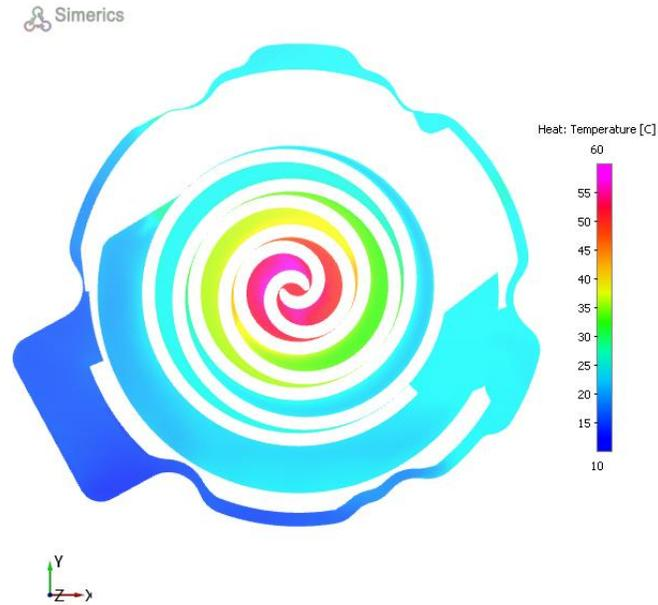
**Figure 11:** Temperature contours on mid-cross section through scroll fluid side for Case 1
