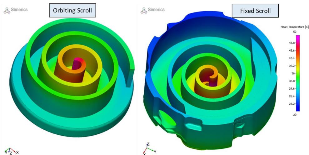
**Figure 13:** Temperature contours on fixed and orbiting scroll for Case 1
