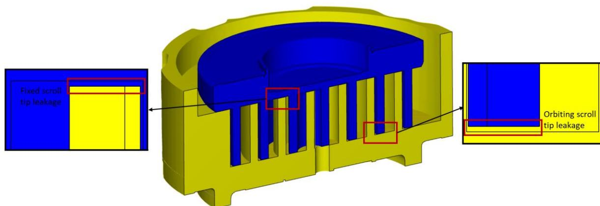
**Figure 5:** Tip leakage (enlarged for viewing) between the fixed (yellow) and orbiting scroll (blue).
