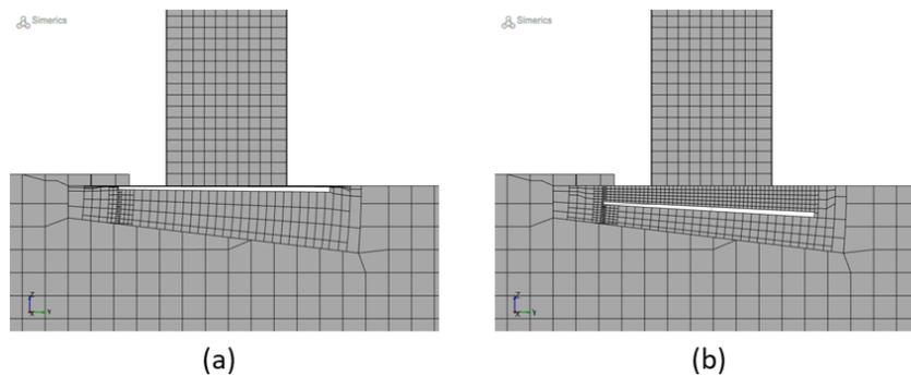
**Figure 2:** Cross-section view of reed valve mesh at (a) closed position and (b) 5° opening
