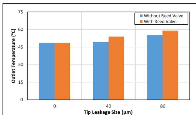
**Figure 17:** Temperature at outlet boundary of E-compressor for different tip leakage sizes
