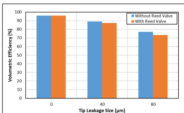
**Figure 16:** Volumetric Efficiency for different tip leakage sizes
