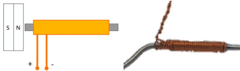
**Figure 1:** Schema of handcrafted inductive sensor (left) and sensor being made (without magnet, right)
