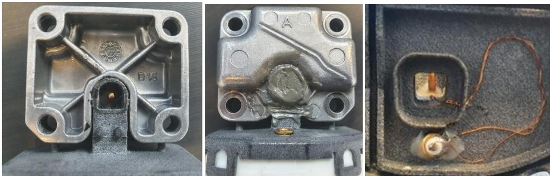
**Figure 3:** Example of headgroup instrumentation of a typical compressor (microdot interface in middle and right pictures)
