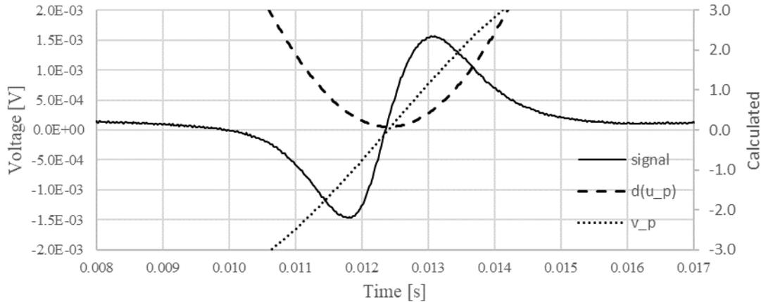
**Figure 7:** Example of measured signal, distance variation between sensor/piston and piston velocity.
