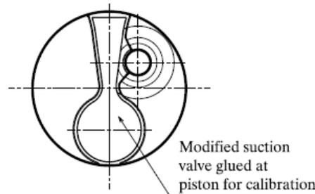
**Figure 6:** Example of position which suction valve should be placed in the piston recess for calibration.
