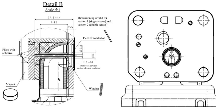
**Figure 2:** Example of instrumentation of a typical compressor's headgroup
