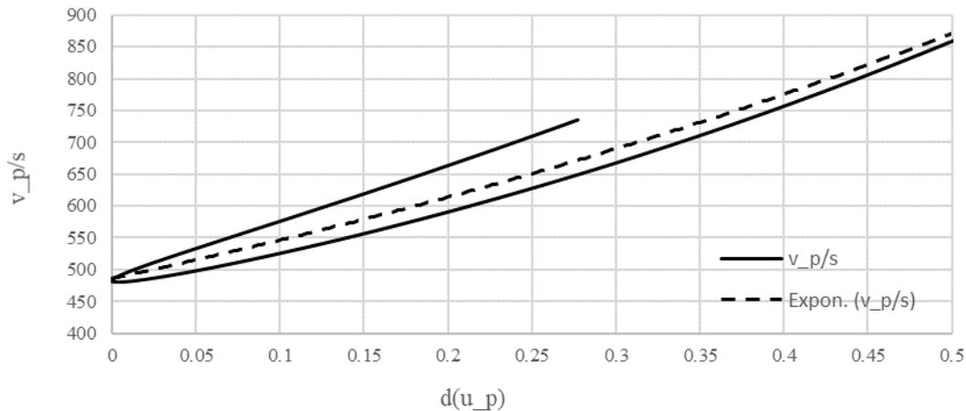
**Figure 8:** Piston velocity/Signal ratio vs. piston displacement when sensor detects movement.
