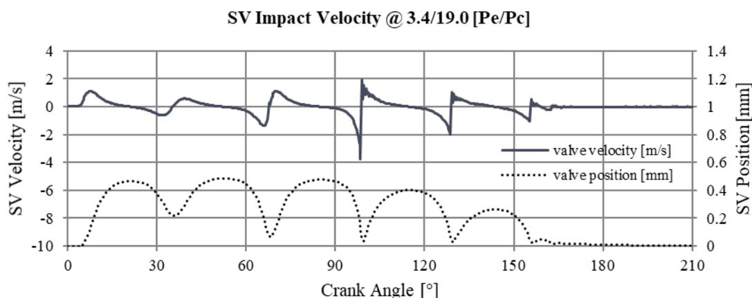
**Figure 9:** Measurement of suction valve impact velocity with 3.4bar pressure on evaporator and 19.0bar pressure on condenser, operating at 3000rpm, using an average  $K_c$  value.
