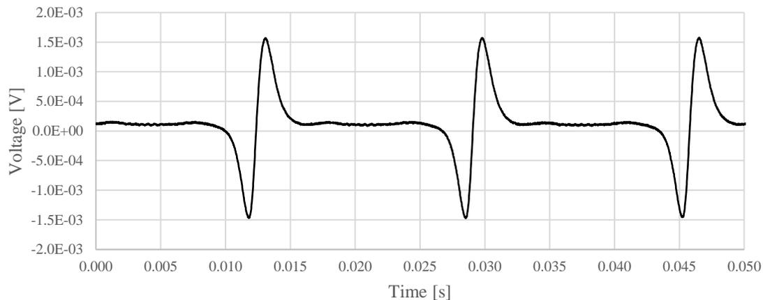
**Figure 5:** Example of a signal acquire from a moving mechanism of a typical compressor.
