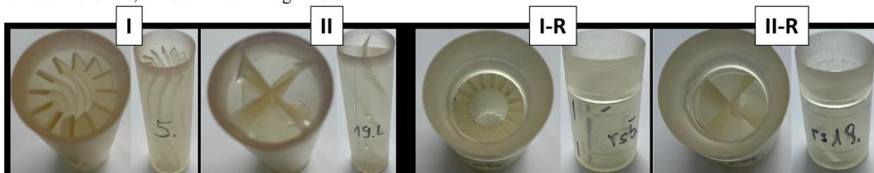
**Figure 6:** 3D printed nozzles for screw compressor manifold. Left – rigid nozzles, right – rotating nozzles
