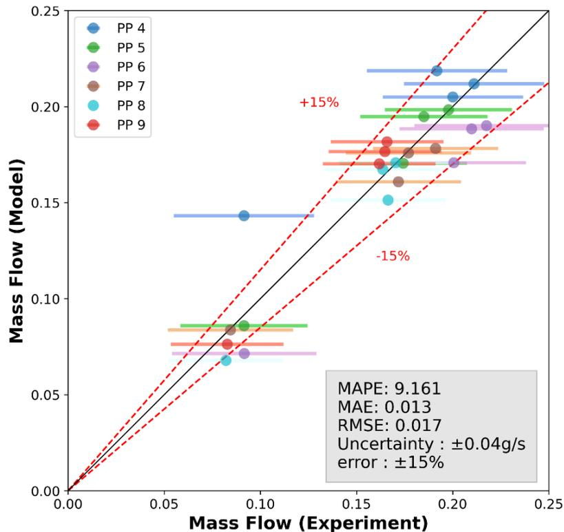
Figure 8: Comparison of experimental and computational mass flow rate.
