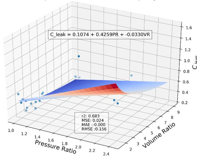
Figure 7: Regression analysis to determine the  $C_{leak}$  relation.
