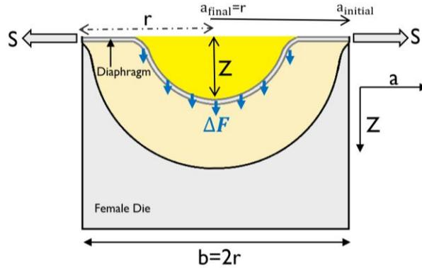
**Figure 2:** Cross-sectional schematic of a compression chamber when piston load deflects the diaphragm.
