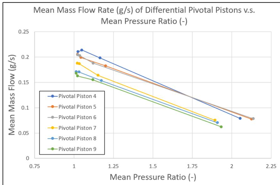
**Figure 6:** Overall repeatability data with mean mass flow plotted as a function of pressure ratio.
