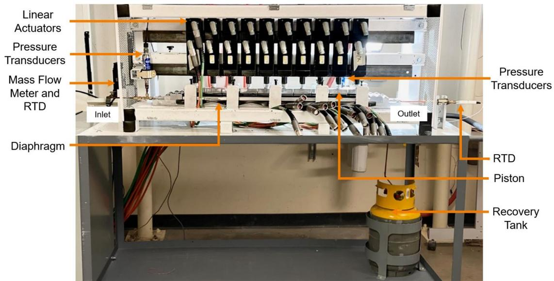
**Figure 5:** Experimental Set up.
