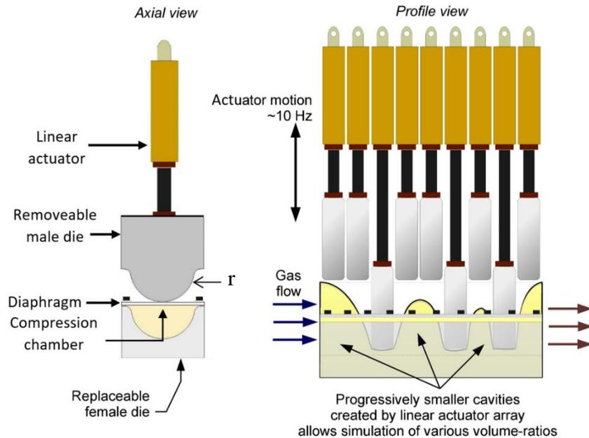
**Figure 1:** A scheme of the proposed reconfigurable peristaltic compressor prototype (Bradshaw, 2017).
