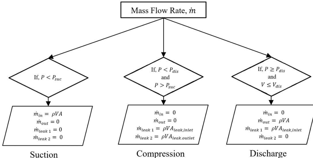
**Figure 4:** Computational algorithm for the mass flow rate.
