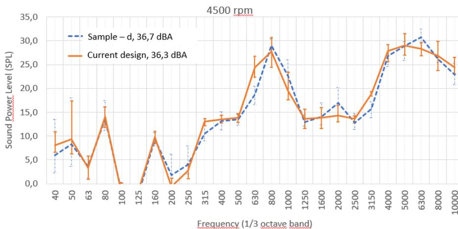
**Figure 13:** Sound power level in 4500 rpm for current design and sample-d
