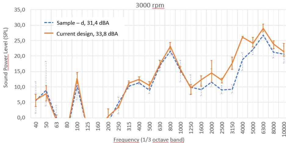
**Figure 12:** Sound power level in 3000 rpm for current design and sample-d
