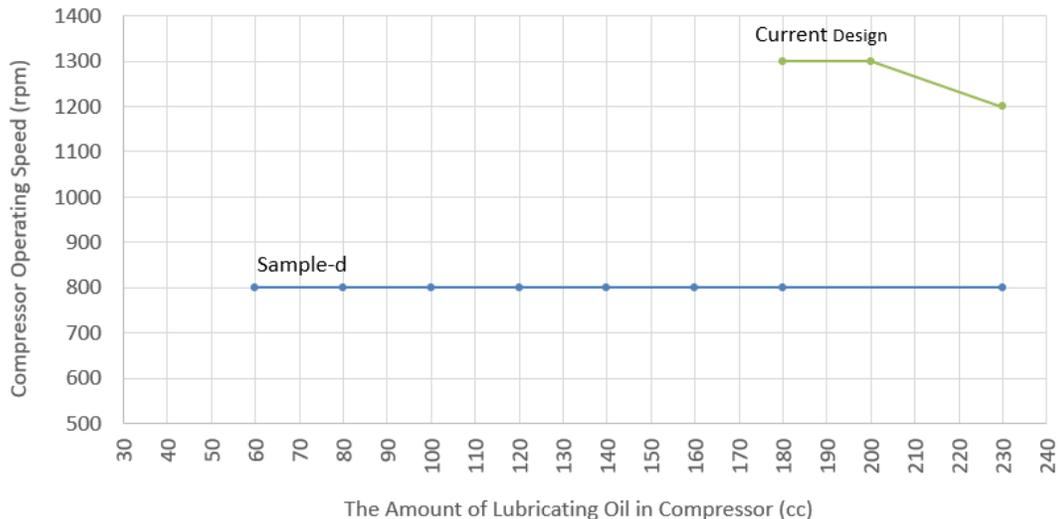
**Figure 9:** Operating speed versus the amount of lubricating oil for current design and Sample-d
