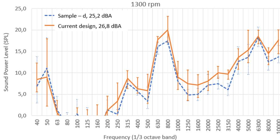
**Figure 11:** Sound power level in 1300 rpm for current design and sample-d
