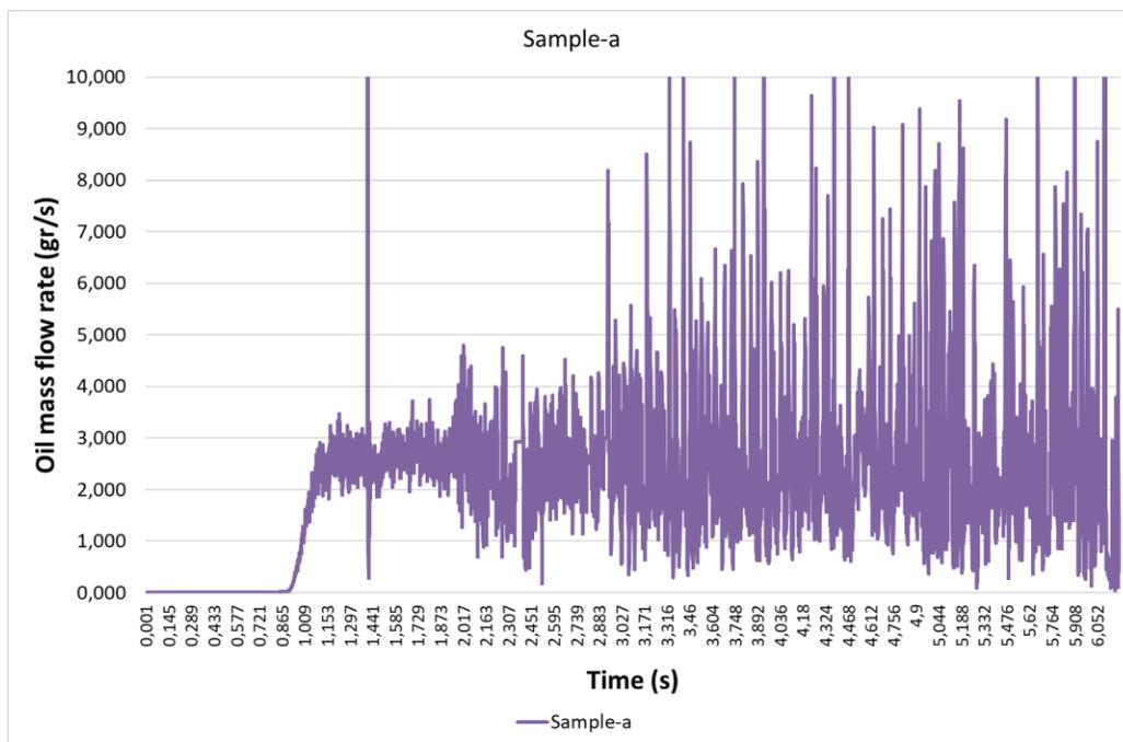
Figure 2: Oil mass flow rate of Sample-a @4500 rpm
