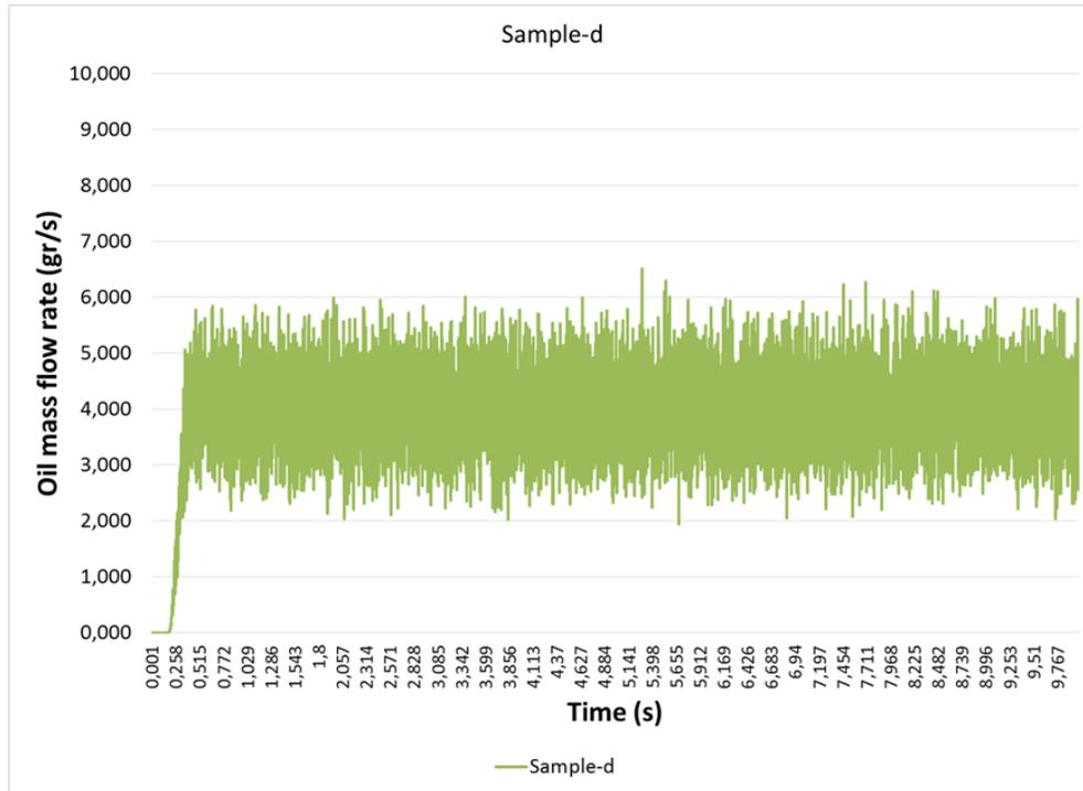
**Figure 5:** Oil mass flow rate of Sample-d @4500 rpm
