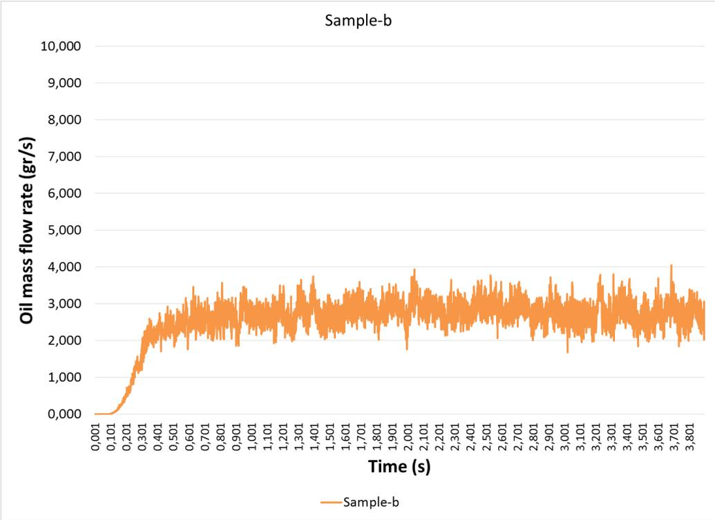
Figure 3: Oil mass flow rate of Sample-b @4500 rpm
