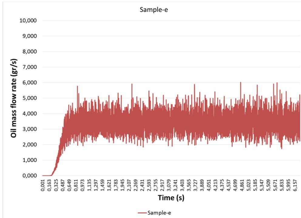
**Figure 6:** Oil mass flow rate of Sample-e @4500 rpm
