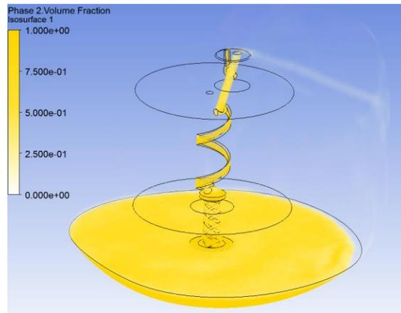
**Figure 7:** CFD Post Process: Volume fraction rendering of compressor oil
