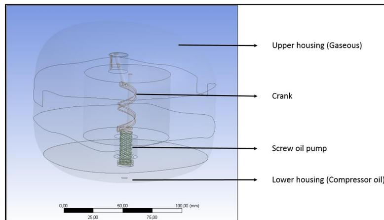
**Figure 1:** Fluid volume of compressor oil system
