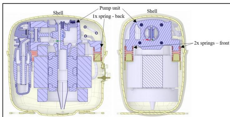
**Figure 1:** Schematic view: compressor with shell, pump unit and springs
