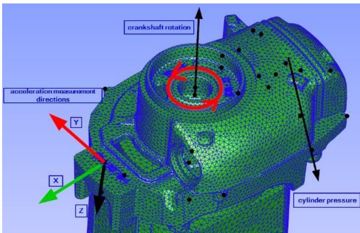
Figure 5: Experimental setup - measured characteristics
