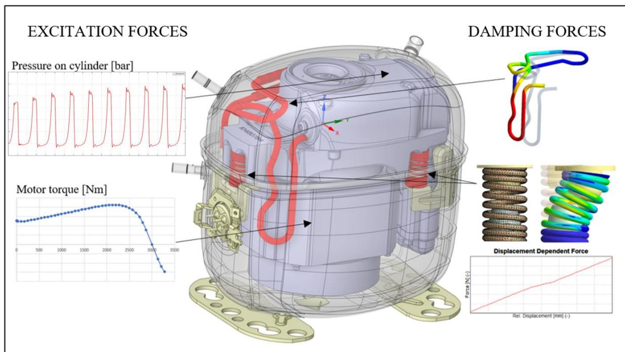
**Figure 2:** Excitation and damping forces affecting pump unit movement
