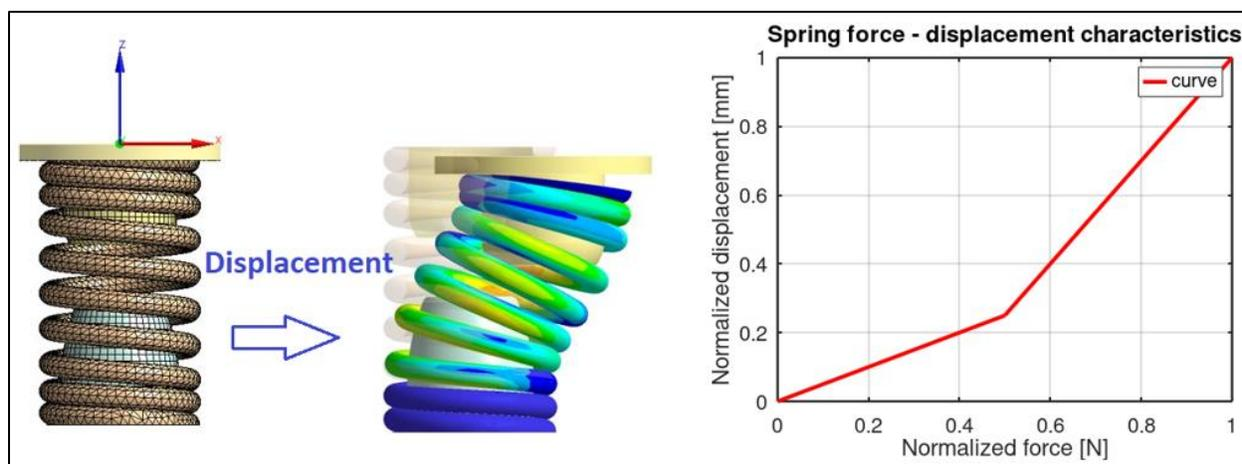
**Figure 4:** Force versus displacement function in a spring
