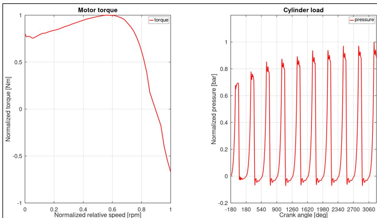
**Figure 3:** Motor torque and cylinder load used for numerical analysis
