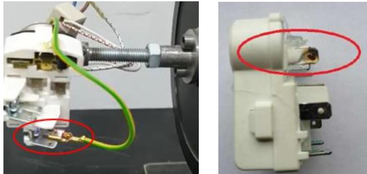
**Figure 2.** Arcing Occurred on Loose Contacts by Applying High Stress Factors
