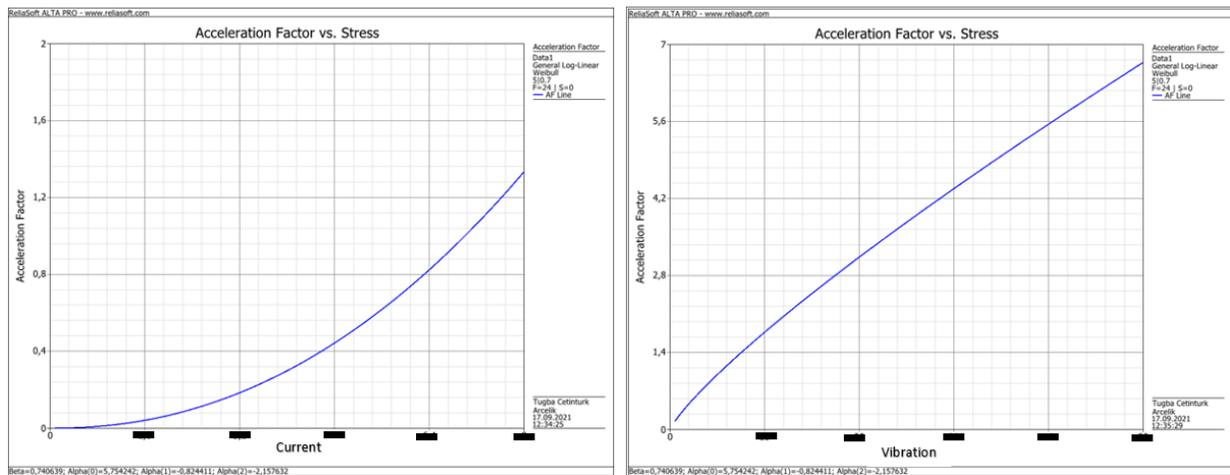
Figure 3. Acceleration Factor vs. Current and Vibration
