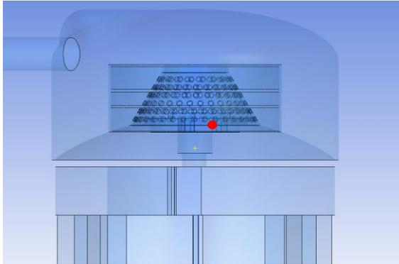
**Figure 10:** Monitor point in compressor
