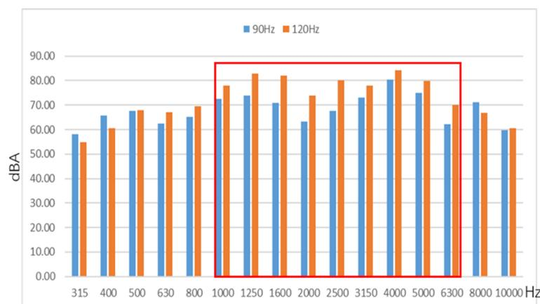
**Figure 2:** Scroll compressor sound power spectrum at 90Hz/120Hz
