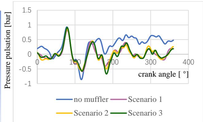
**Figure 11:** Pressure pulsation comparison curve
