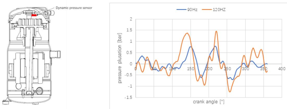
**Figure 5:** Discharge port dynamic pressure pulsation curve
