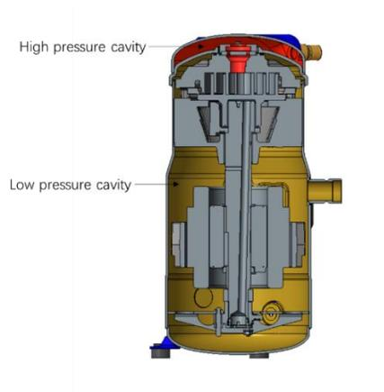
**Figure 1:** Typical Danfoss Scroll compressor cross section
