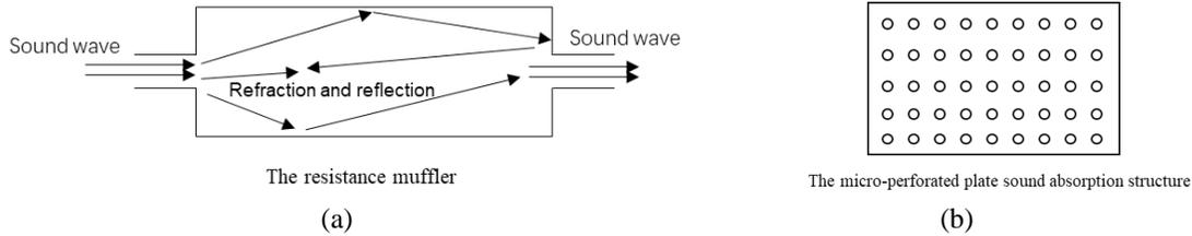
**Figure 6:** Different muffler types
