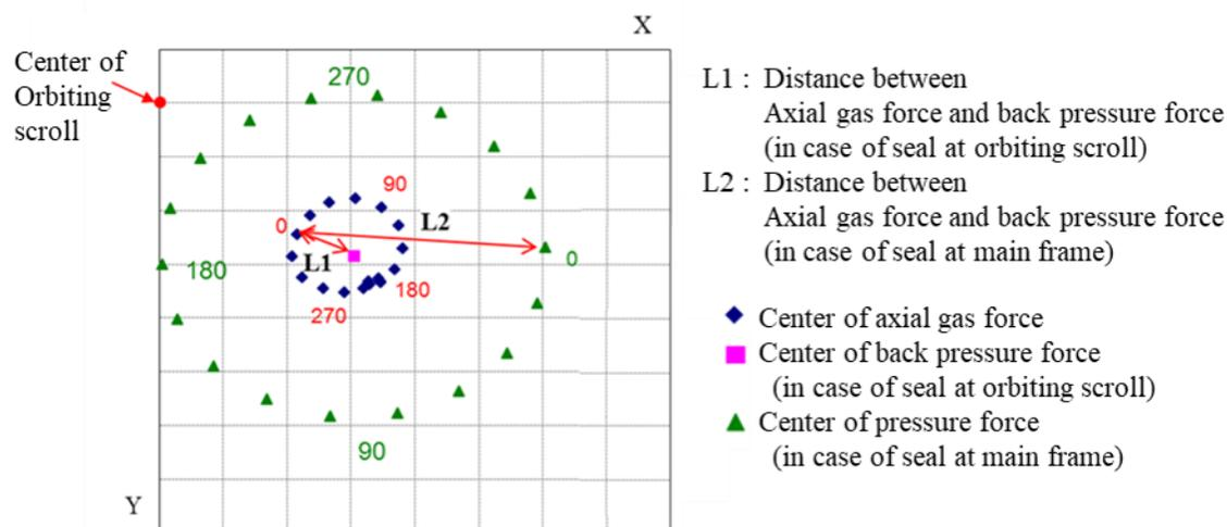
**Figure 10:** Force action point according to position of backpressure seal
