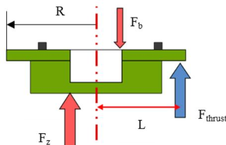
Figure 9: Axis direction force of orbiting scroll
