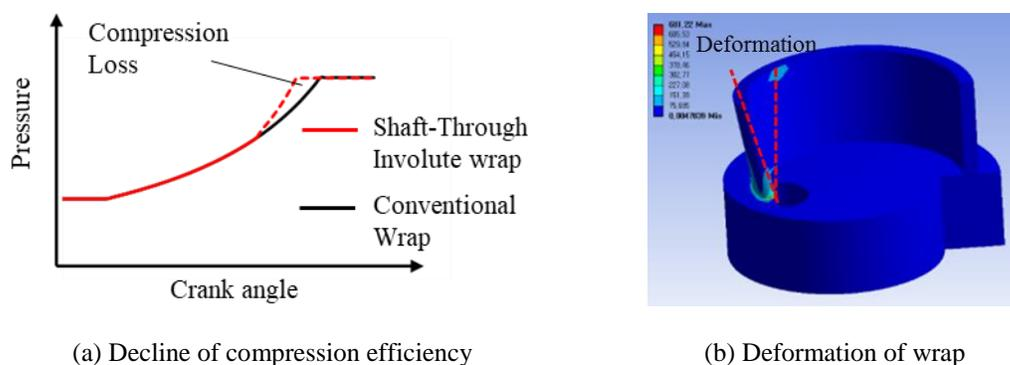
**Figure 3:** Problems of conventional involute scroll wrap with shaft through structure
