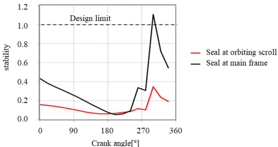
**Figure 11:** Comparison of stability according to position of back pressure seal
