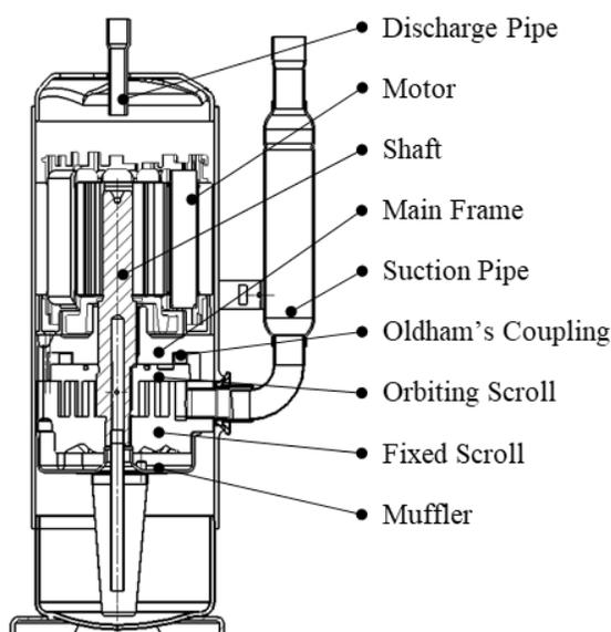
**Figure 1:** Cross sectional view of the R1 compressor
