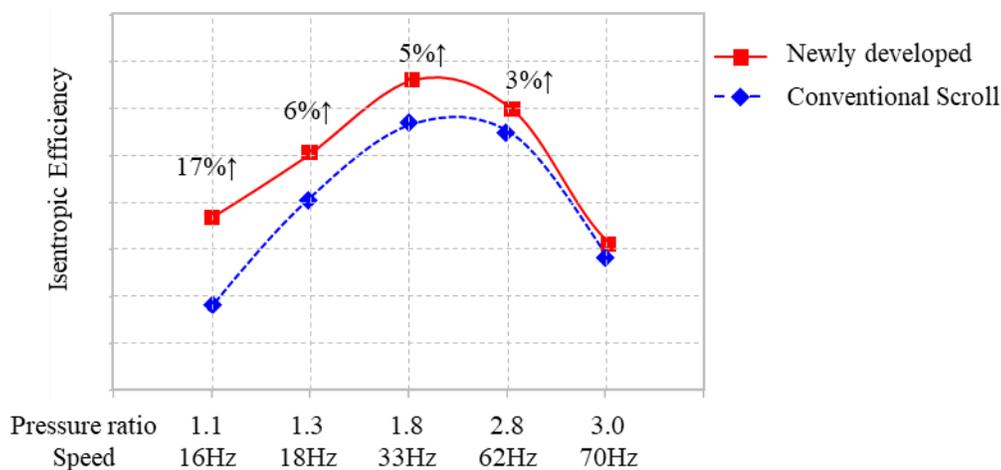
**Figure 15.** Comparison of efficiency with the scroll compressor
