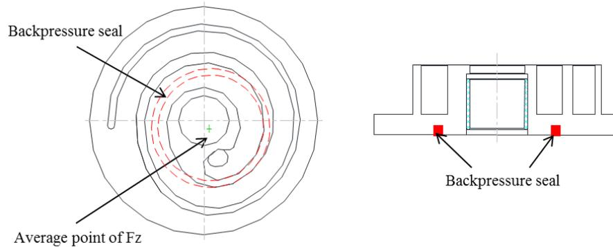
**Figure 12:** Eccentric back pressure seal
