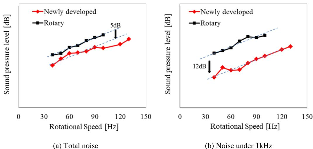
**Figure 16.** Comparison of sound pressure level
