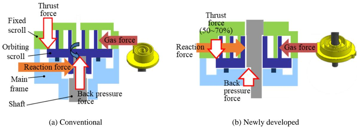
Figure 8: Position of reaction force
