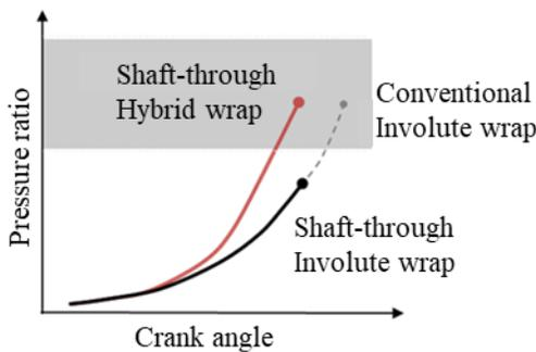
Figure 5: Pressure ratio of the new shape scroll wrap
