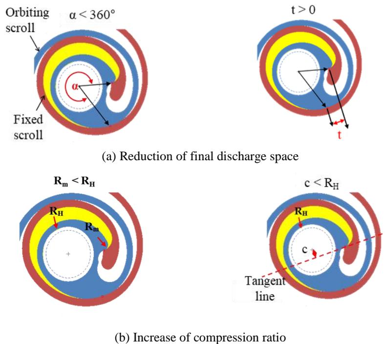
Figure 4: Design of the new shape scroll wrap using hybrid wrap
