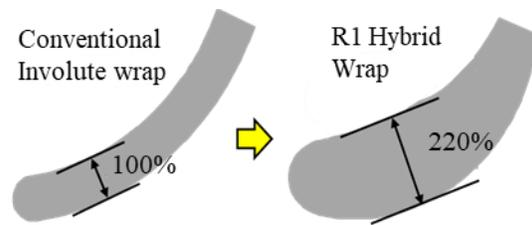
Figure 6: Thickness of center wrap
