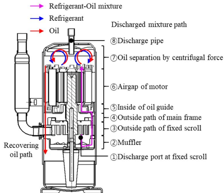
**Figure 13:** circulated path of the oil and refrigerant
