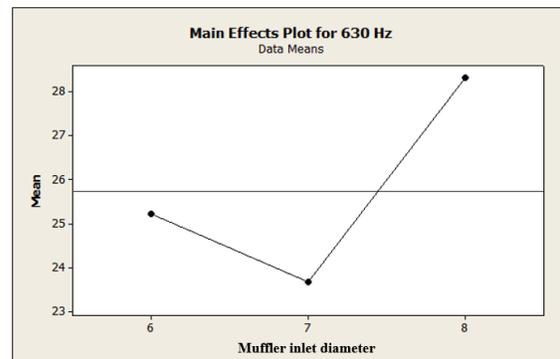
**Figure 11:** The change on the noise level (630Hz) of the compressor for experiments
