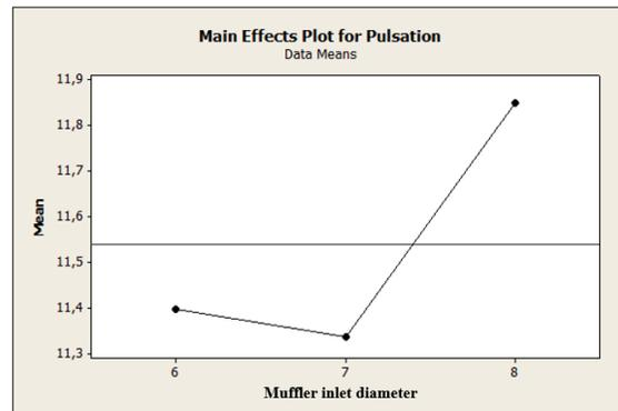
**Figure 10:** The change on the pulsation of the compressor for experiments
