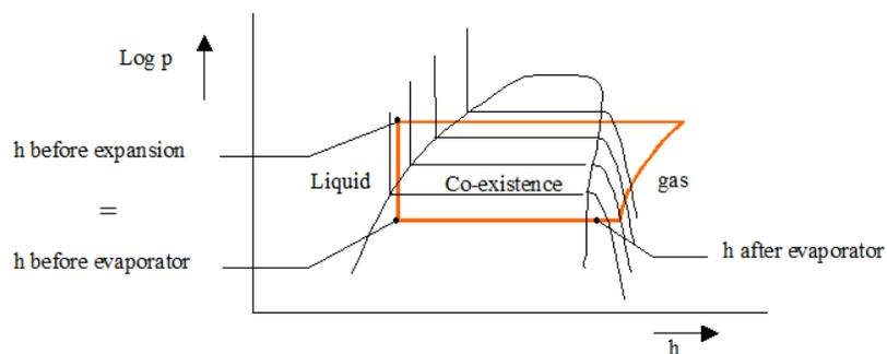
**Figure 4:** Cooling capacity determination
