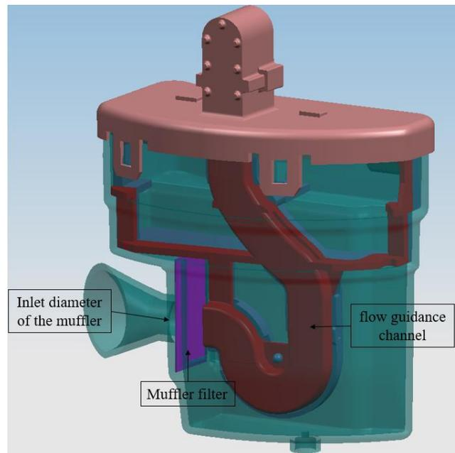
**Figure 3:** The inlet diameter, muffler filter and flow guidance channel of the suction muffler
