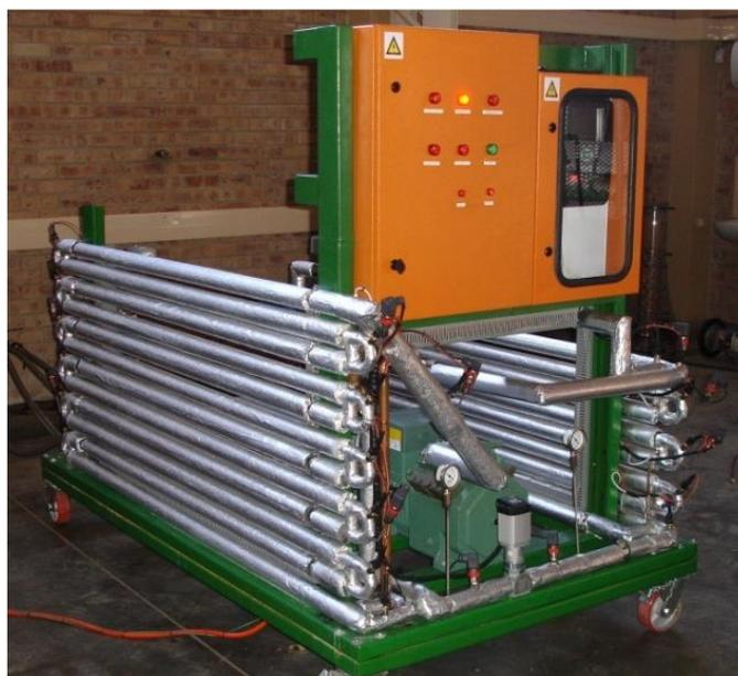
Figure 2: Experimental heat pump test bench with a Bitzer JTC-15K reciprocating, semi-hermetic CO<sub>2</sub> compressor.
