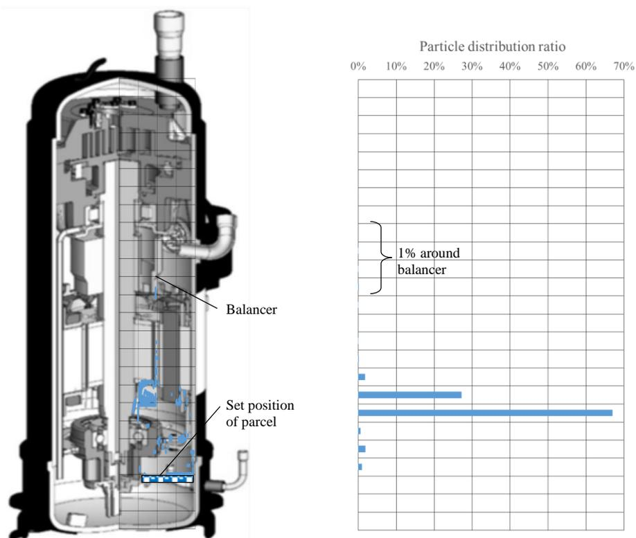
Fig. 5: Particle flow from the oil pool in the bottom of the scroll compressor at 130[rps]
