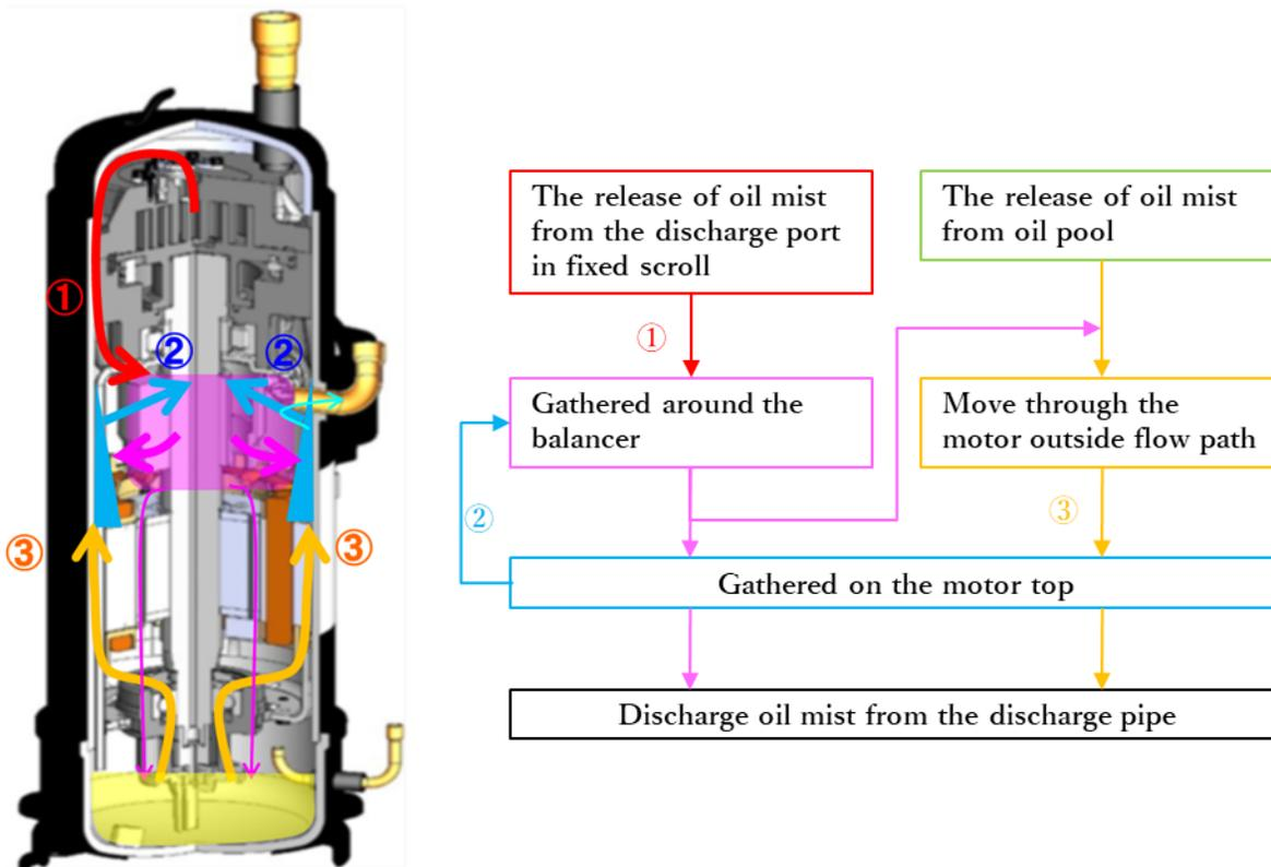
Fig. 6: Mechanism of Oil mist behavior in the scroll compressor
