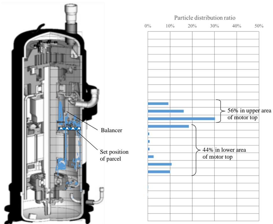
Fig. 4: Particle flow from the motor top at 130[rps]
