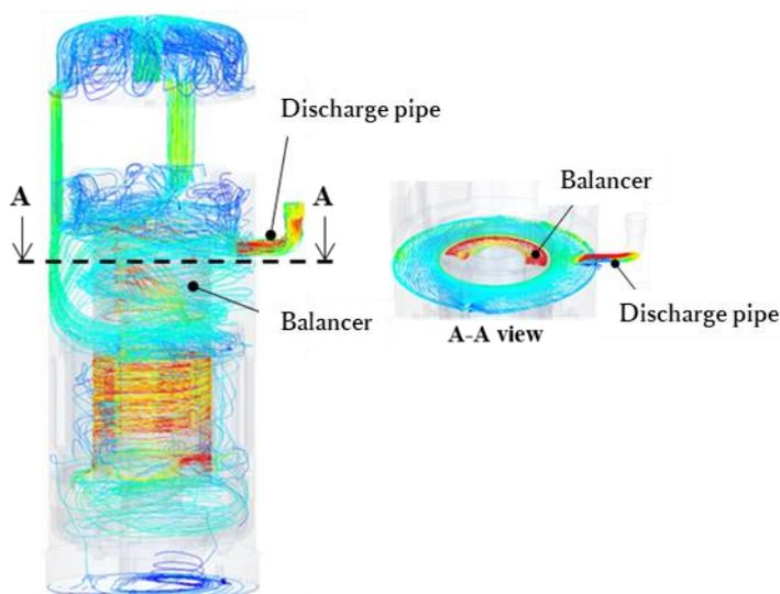
**Fig. 2:** Refrigerant flow in the scroll compressor at 130[rps]
