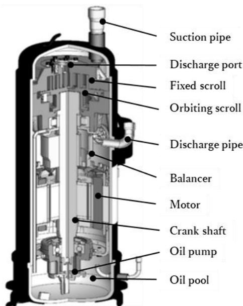
**Fig. 1:** Cross section of the scroll compressor
