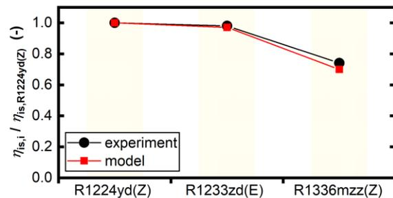
**Figure 4:** Calculated (squares) and measured (circles) rel. isentropic compressor efficiencies for DS4. Calculated using  $a_{scale}$ ,  $b_{scale}$ ,  $c_{ref}$ ,  $k_{1,ref}$ ,  $k_{2,ref}$  and the respective measured inlet and outlet states.  $T_{evap} \approx 25\text{ }^{\circ}\text{C}$ ,  $T_{cond} \approx 70\text{ }^{\circ}\text{C}$ ,  $T_{in} \approx 50\text{ }^{\circ}\text{C}$ .
