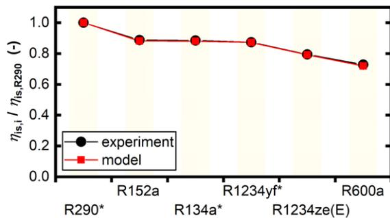
**Figure 3:** Calculated (squares) and measured (circles) rel. isentropic compressor efficiencies for DS3. Calculated using  $a_{scale}$ ,  $b_{scale}$ ,  $c_{ref}$ ,  $k_{1,ref}$ ,  $k_{2,ref}$  and the respective measured inlet and outlet states.  $T_{evap} \approx 0\text{ }^{\circ}\text{C}$ ,  $T_{cond} \approx 35\text{ }^{\circ}\text{C}$ ,  $T_{in} \approx 12\text{ }^{\circ}\text{C}$ .
