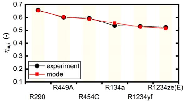
**Figure 1:** Calculated (squares) and measured (circles) isentropic compressor efficiencies for DS1. Calculated using fitted  $a_{ref}$ ,  $b_{ref}$ ,  $c_{ref}$ ,  $k_{1,ref}$ ,  $k_{2,ref}$ .  $T_{evap} = 0\text{ }^{\circ}\text{C}$ ,  $T_{cond} = 35\text{ }^{\circ}\text{C}$ ,  $T_{in} = 20\text{ }^{\circ}\text{C}$ .
