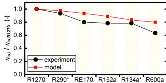
**Figure 2:** Calculated (squares) and measured (circles) rel. isentropic compressor efficiencies for DS2. Calculated using  $a_{scale}$ ,  $b_{scale}$ ,  $c_{ref}$ ,  $k_{1,ref}$ ,  $k_{2,ref}$  and the respective measured inlet and outlet states.  $T_{evap} \approx 0\text{ }^{\circ}\text{C}$ ,  $T_{cond} \approx 33\text{ }^{\circ}\text{C}$ ,  $T_{in} \approx 17\text{ }^{\circ}\text{C}$ .
