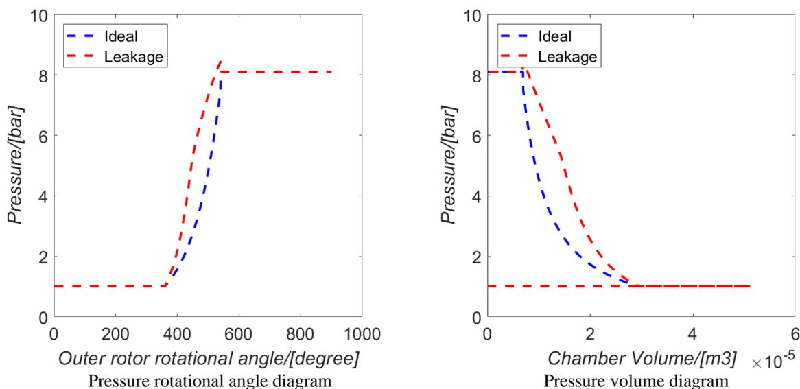
**Figure 7:** Pressure diagram
