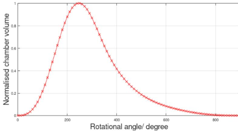
**Figure 3:** Chamber volume changing with rotational angle
