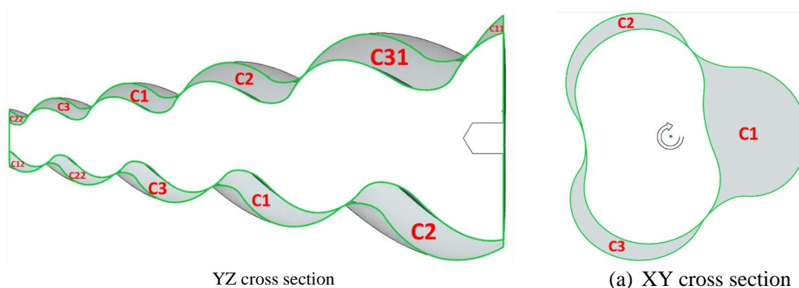
**Figure 5:** Rotor cross sections to show leakage paths
