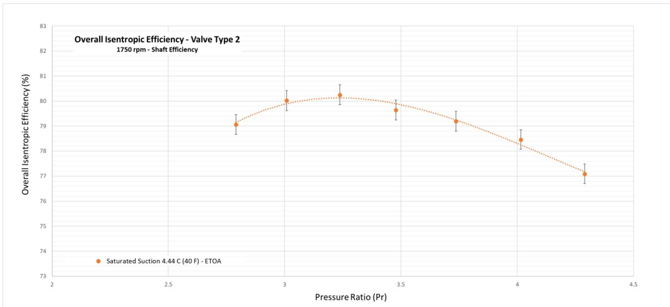
Figure 7: 106 kW spool compressor overall isentropic efficiency ( $\eta_{is,0}$ ) vs. pressure ratio at 1750 rpm – Valve Type 2
