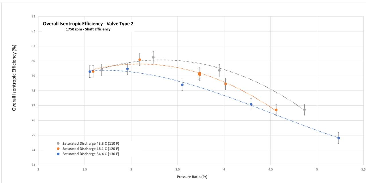
Figure 8: 106 kW spool compressor all isentropic efficiency ( $\eta_{is,0}$ ) Multiple condensing temperatures at 1750 rpm – Valve Type 2
