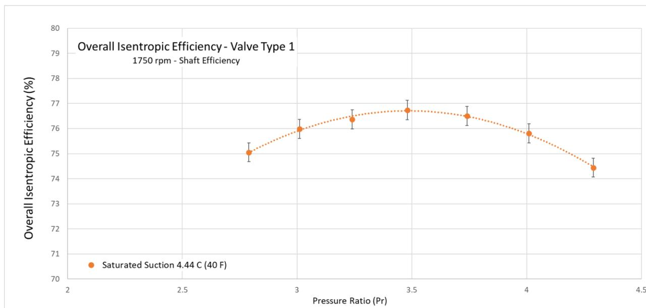
Figure 6: 106 kW spool compressor overall isentropic efficiency ( $\eta_{is,0}$ ) vs. pressure ratio at 1750 rpm – Valve Type 1
