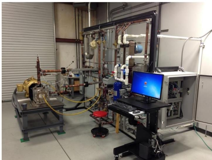
Figure 2: Photo of 141 kW hot gas bypass test stand
