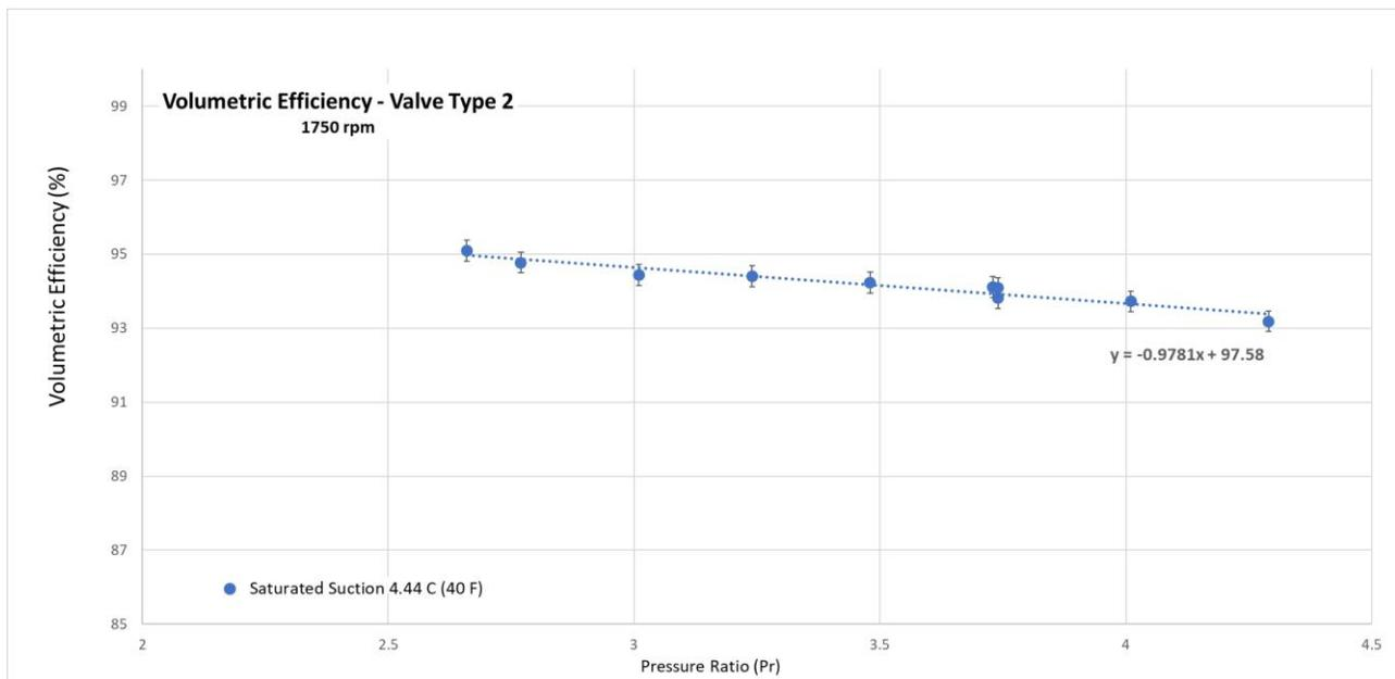
Figure 5: 106 kW spool compressor volumetric efficiency vs. pressure ratio at 1750 rpm – Valve Type 2.
