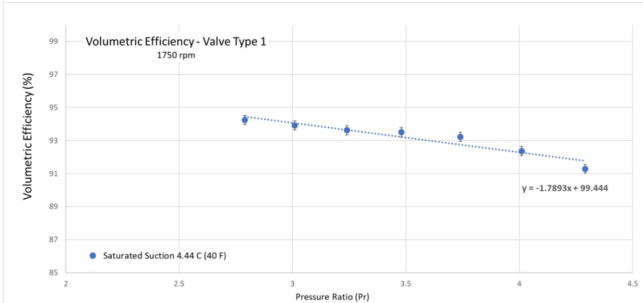
Figure 4: 106 kW spool compressor volumetric efficiency vs. pressure ratio at 1750 rpm – Valve Type 1.
