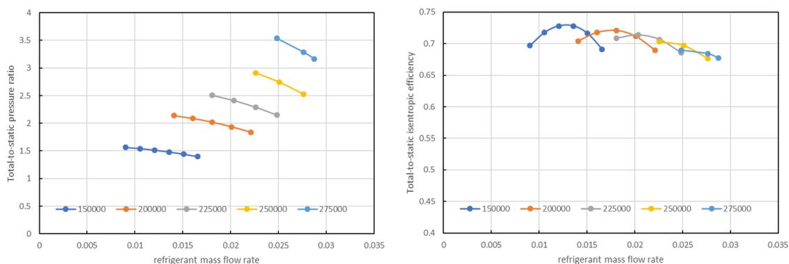
**Figure 3:** Compressor performance map - optimized design: (left) pressure ratio, (right) efficiency.
