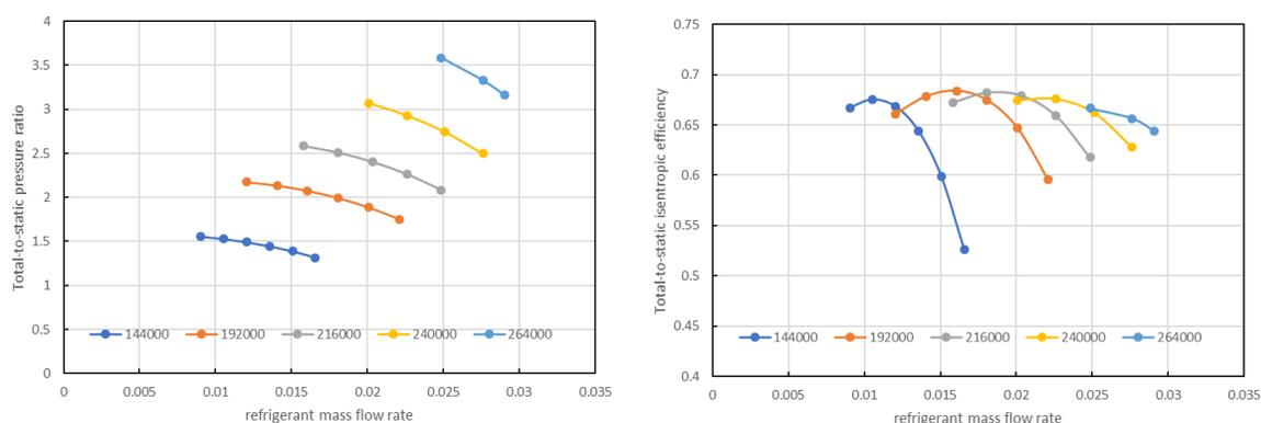
**Figure 2:** Compressor performance map - base design: (left) pressure ratio, (right) efficiency.
