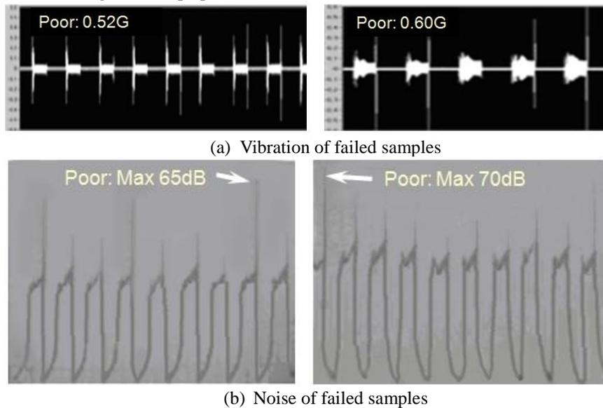
**Figure 7:** The vibration and noise of failed compressors in 1<sup>st</sup> ALT
